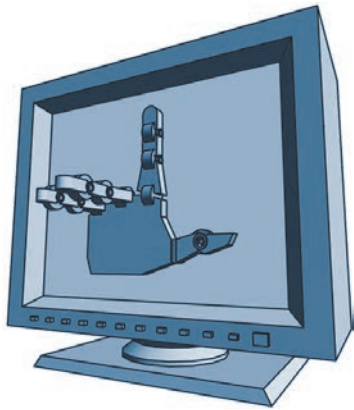
4.2 The Z-Axis. In systems that use the right-hand rule, the positive Z-axis points toward you when the face of the monitor is parallel to the X-Y plane.
