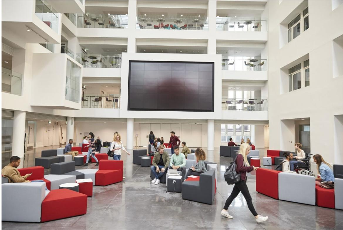
Figure 7-6 An atrium is an open space with no attenuation connecting several floors, a Wi-Fi interference nightmare
