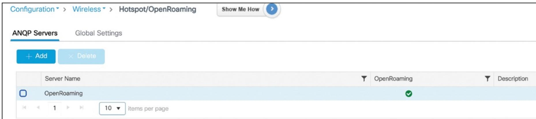
Figure 11-16 WLC OpenRoaming configuration page
