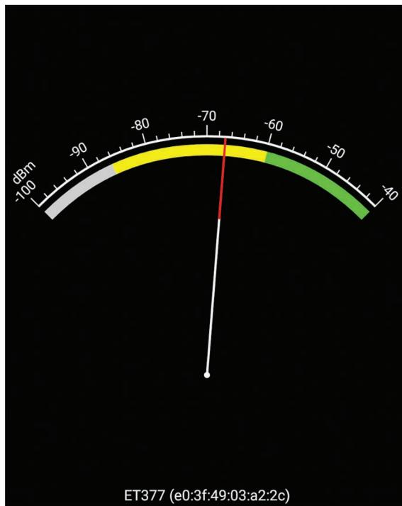
**FIGURE 4-16** The drop in the signal quality to fair at point C.
