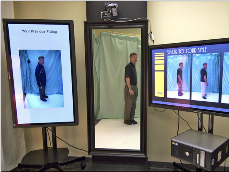
Figure 11-2 The Responsive Mirror prototype. The images in the left display show previous clothing trials matching the same pose in real time as the person turns in the mirror. The images in the right display also match the pose but show other clothing similar to what the shopper is trying on.
