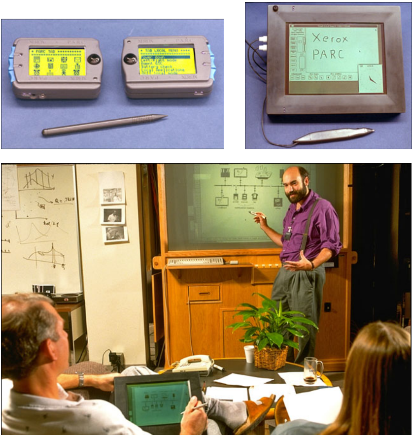
Figure 2-1 Early examples of Ubiquitous Computing devices circa 1991: PARC Tab handheld computer (upper left), PARC Pad tablet computer (upper right), and Liveboard wall-sized computer (bottom). © Palo Alto Research Center, Inc. Included here by permission.
