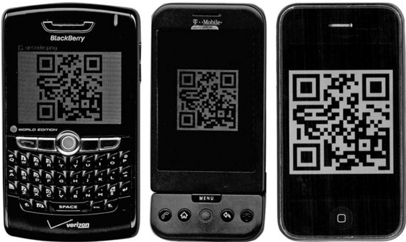
Figure 9-2 Sample scans of QR codes by different models of printer/copiers and smartphones. (Image credit: Hua Liu and Arturo Lorenzo)
