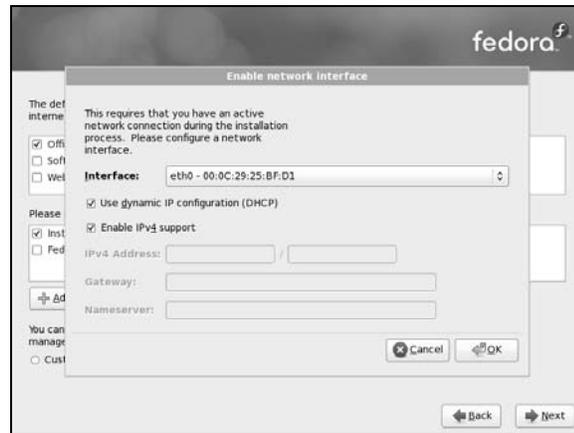
**Figure 3-10** The Enable Network Interface window
