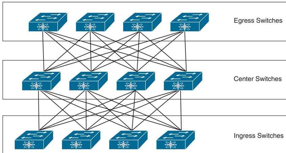
**Figure 2-1** *Conceptual View of a Three-Stage Clos Topology*
