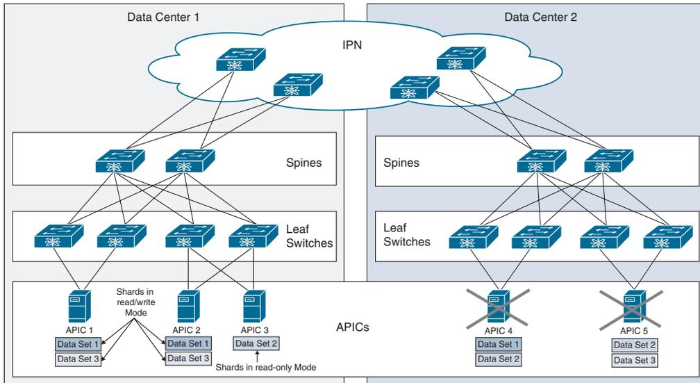
**Figure 2-11** *Impact of APIC Failures in a Five-Node Cluster*
