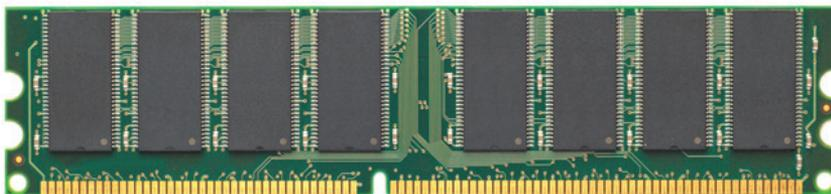
**Figure 2-18** RAM Stick (the Notch in the Bottom Helps Installation Orientation)
