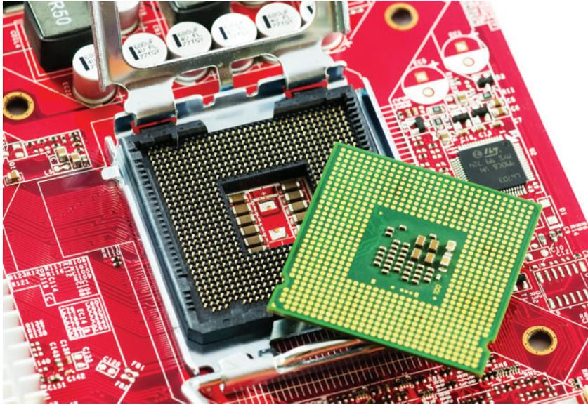
**Figure 2-17** LGA CPU and LGA Motherboard Socket (the Pins Are on the Motherboard)
