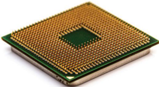
**Figure 2-16** PGA CPU (the Pins Are on the CPU)
