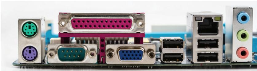
**Figure 2-10** *Directly Below the Large Pink Parallel Port Is a Serial Port (Left) and a Blue VGA Port (Right)*
