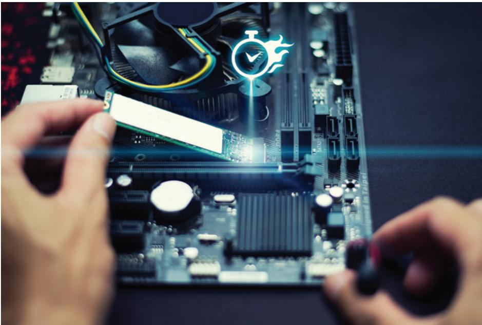
**Figure 2-21** M.2 NVMe Drive Being Installed
