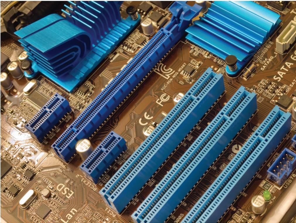
**Figure 2-22** PCIe Expansion Slots (Bottom Three Are Older PCI Slots; Above Bottom Three Is PCIe x1, Followed by PCIe x16, and Top Is PCIe x1)
