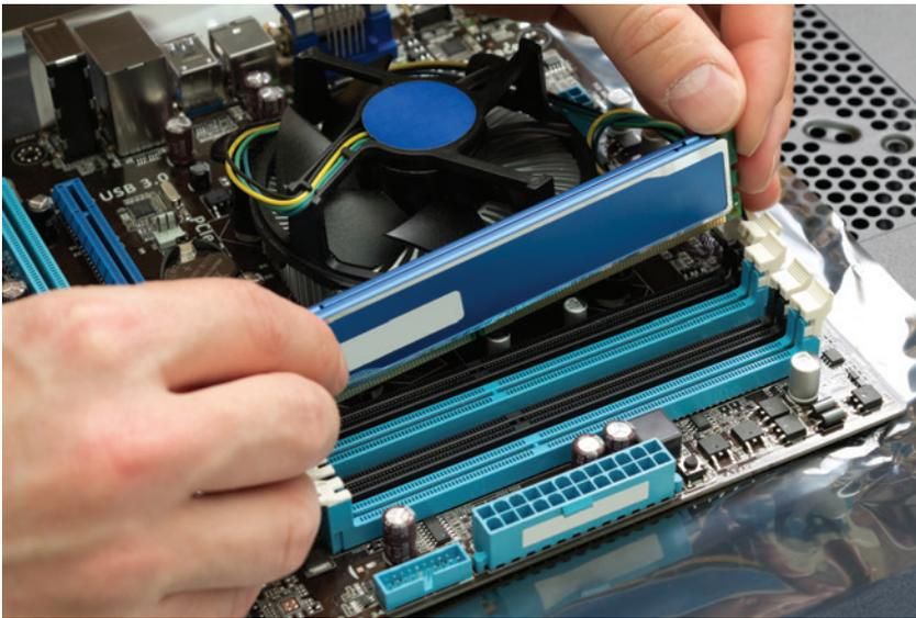
**Figure 2-19** *DIMM Slots with Color-Coded Channels*
