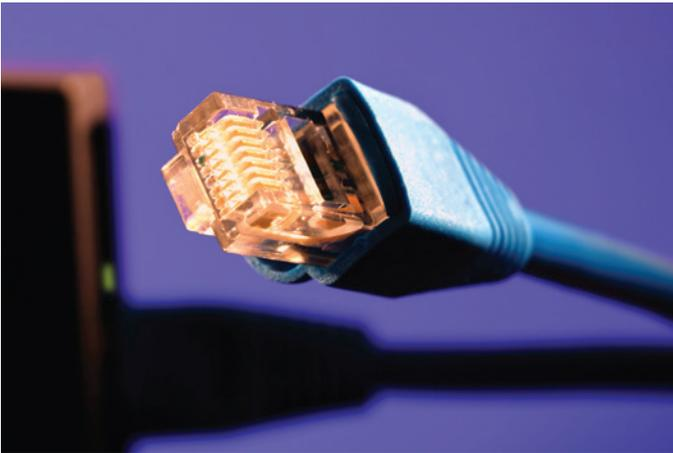
**Figure 2-13** RJ-45 Connector (Wider and Has More Wires Than the Older Telephone Connector, Which Was an RJ-11)
