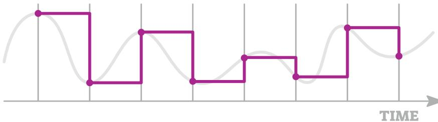
**Figure 2-4** Analog vs. Digital Signal
