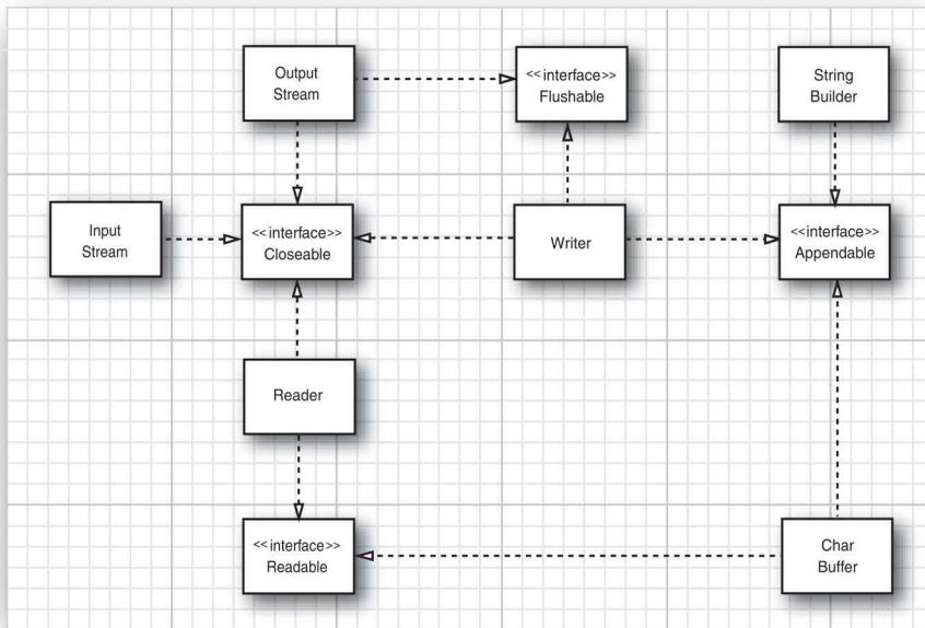
**Figure 2.3** The Closeable, Flushable, Readable, and Appendable interfaces
