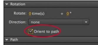
Animate inserts keyframes for rotation along the motion tween to orient the nose of the rocket ship to the path of the motion.
