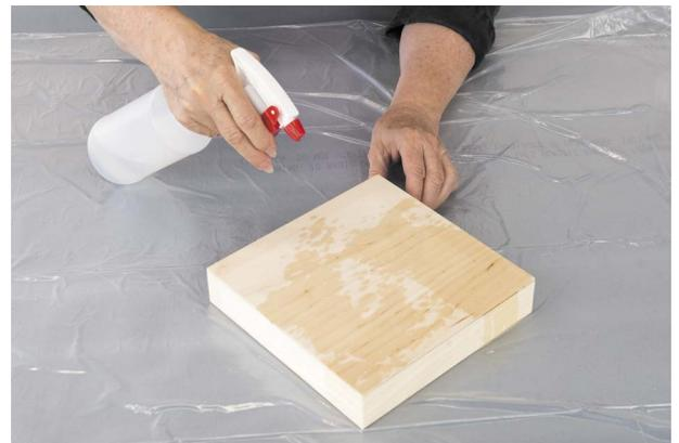
**FIGURE B.3** Wetting the wood raises the grain for sanding so it won't raise again later.
