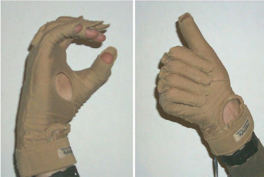
**Figure 9.11** Examples of postures using a Data Glove. (Photograph courtesy of Joseph J. LaViola Jr.)
