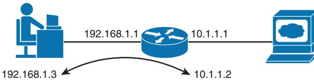
As shown in Figure 3-3, use an extended **ping** or **tracert** to originate traffic from the 10.1.1.1 interface to check connectivity. If possible, examine neighboring devices to determine whether their routing tables include the return route to 10.1.1.0/24.
