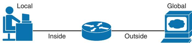
NAT can map addresses to pool or to a single address. Mapping all the inside connections to a single public address is an example of Port Address Translation (PAT) or overloading.
