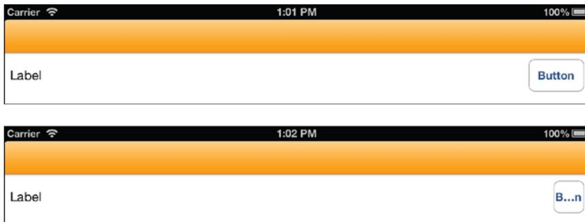
**Figure 1-10** Compression resistance describes how a view attempts to maintain its minimum intrinsic content size. The top screenshot's button has a high compression resistance.
