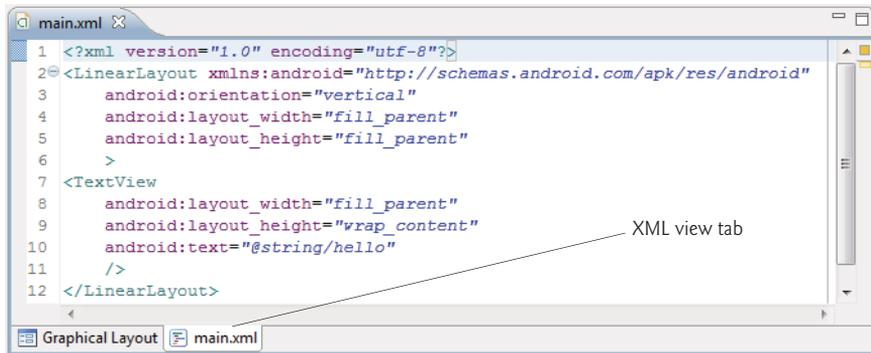
**Fig. 3.8** | XML view of the app's default GUI.
