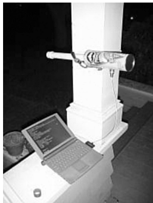
Figure 8-4 Pringles Can as a Yagi Antenna
