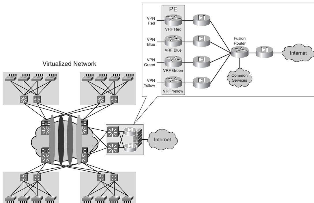
As shown in Figure 3-8, each VN is head ended by a dedicated firewall. This allows the creation of security policies specific to each VN and independent from each other. To access the shared services, all firewalls are connected to a “fusion” router. The fusion router can provide the VNs with connectivity to the common services, the Internet, or even inter-VN connectivity. The presence of this fusion router should raise two main concerns:
