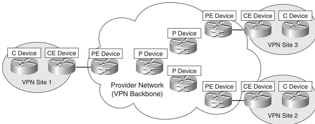
In Layer 2 VPNs, such as a Virtual Private LAN Service (VPLS), an additional level of hierarchy can be introduced into the network to improve scalability (VPLS then becomes Hierarchical VPLS [H-VPLS]). In this case, the functionality of the PE device is divided between a User-facing PE (U-PE) devices and Network-facing PE (N-PE) devices.
