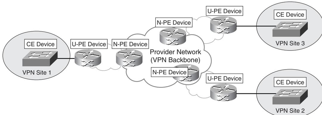
Other device types used in VPNs include Network Access Servers (NAS) and VPN gateways/concentrators. A NAS is a device that interfaces between an access network (such as a Public Switched Telephone Network [PSTN]) and a packet-switched network (such as an IP backbone). In a remote access VPN, a NAS can serve as a tunnel endpoint.
