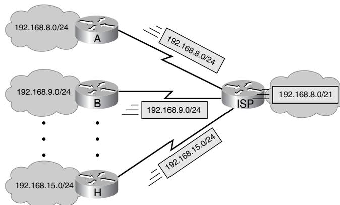
The mechanism used to calculate the summary route to advertise is the same as shown in the “Route Summarization” section. The Class C network addresses 192.168.8.0/24 through 192.168.15.0/24 are being used and are being advertised to the ISP router. To summarize these addresses, find the common bits, as shown here (in bold):
