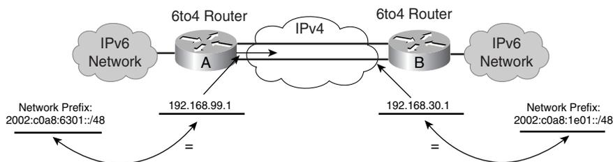
The 6to4 tunneling method requires configuration of the edge routers, but the IPv6 hosts and routers inside the 6to4 site do not require new features to support 6to4.
