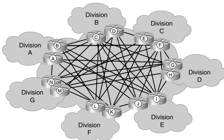
For a small core with a limited number of divisions, this core layer design provides robust connectivity. However, a fully meshed core layer design is very expensive for a corporation with many divisions.
