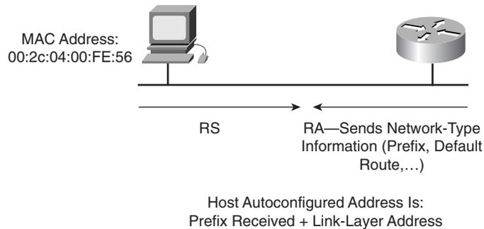
Routers also send RAs periodically, upon request, on all their configured interfaces. The router sends an RA to the *all-nodes* multicast address. Information contained in the RA message includes the following:
