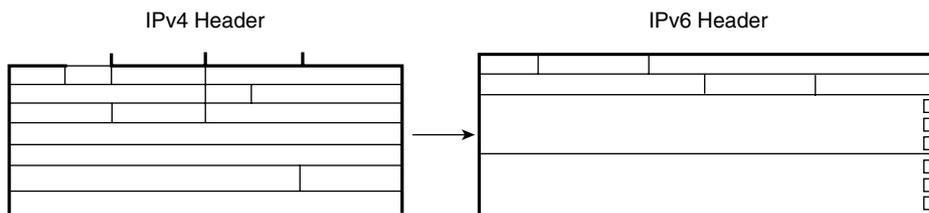
IPv6 header enhancements enable hardware-based processing that provides forwarding rate scalability for the next generation of high-speed lines. In the long term, it is clear that IPv6 improves routing efficiency. In the short term, however, the impact of the larger, 128-bit addressing remains unclear.
