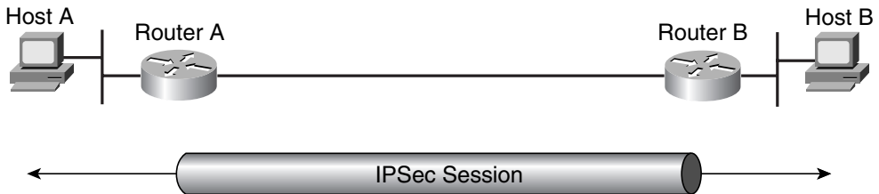
Figure 1-27 Step 4: IPSec Data Transfer
