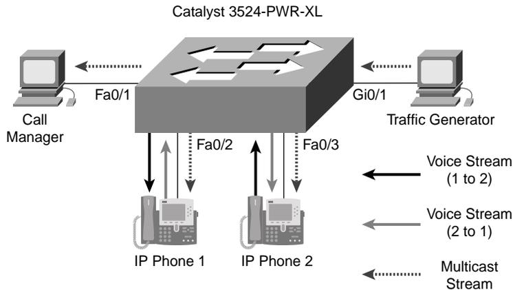
The Catalyst 3524XL switch was running software version 12.0(5)WC5 for the trial. The configuration only included voice VLANs on the Cisco IP Phone ports. The remaining port configuration of the switch was default. Example 3-3 shows the relevant configuration.
