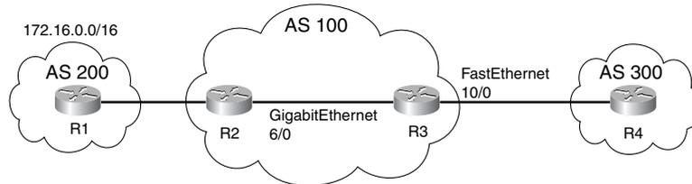
Example 4-31 shows a sample BGP configuration on R3. The router number is used as the host address. The route map Set-policy sets the FIB QoS-group ID to 2 for prefixes matching the community 100:200, which is tagged for 172.16.0.0/16 by R2.
