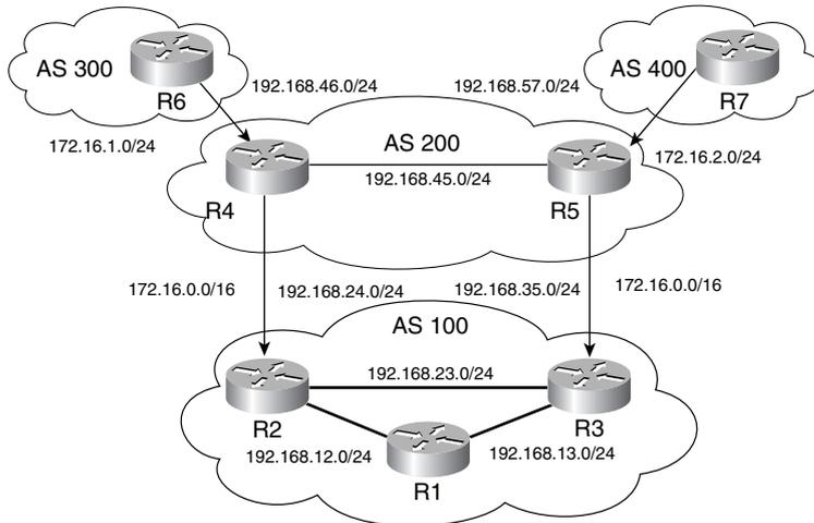
With traffic statistics analysis, AS 100 determines that the best exit for 172.16.1.0/24 is via R2. It is also found that the best exit to 172.16.2.0/24 is via R3. In an effort to optimize the exit points, conditional injection is deployed on R2 and R3. The network address for each link is specified in Figure 4-4, with each router's number as the host address.
