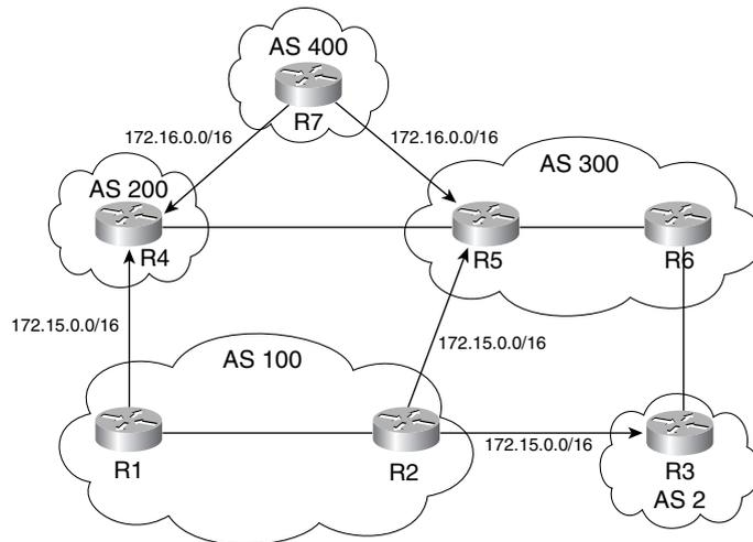
For the purposes of this case study, the last octet of an IP address indicates the router number. Basic BGP configurations for R1 and R2 are shown in Examples 4-40 and 4-41, respectively.
