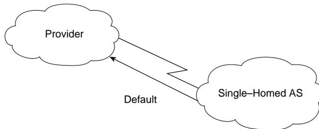
A single-homed AS does not really have to learn Internet routes from its provider. Because there is a single way out, all traffic can default to the provider. When using this configuration, the provider can use different methods to advertise the customer's routes to other networks.
