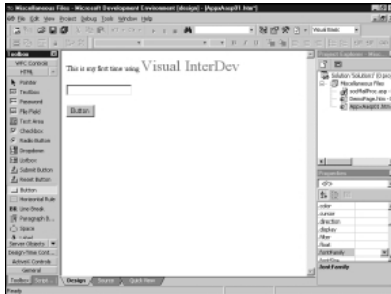
Figure 11: Visual InterDev allows you to add HTML elements to your HTML documents in Design view by dragging and dropping or by double-clicking element icons in the toolbox, just as you did in Source view.
