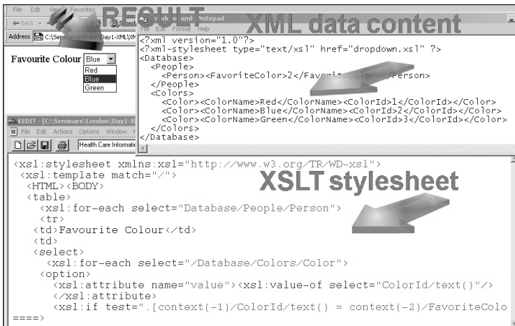
Figure 4.3 How a style sheet works to display XML as HTML.
