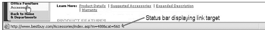
FIGURE 4-4 CGI parameters in the status bar when a user hovers over a link.
