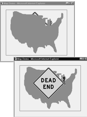
Figure 17.7 The timeline changes the Z-index of the layers. In the first screen, the layers “person” and “deadend” are stacked behind “map.” In the second screen, the map layer has the lowest z-index and is thus stacked behind the other two.
