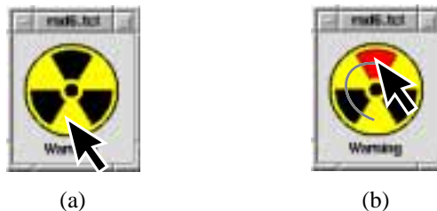
Figure 4.8. Detecting the current item. (a) The pointer is on the canvas. (b) The pointer moves onto an item with the tag name hilite , but this time only the current item changes color.
