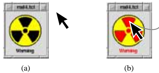
Figure 4.6. Binding to the canvas as a whole. (a) The pointer is outside the canvas. (b) The pointer moves inside the canvas and the items tagged as hilite change color.
