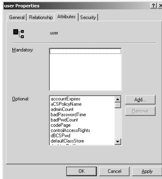
FIGURE 8.14 The Attributes tab lists the mandatory and optional attributes for the class, excluding inherited attributes.
