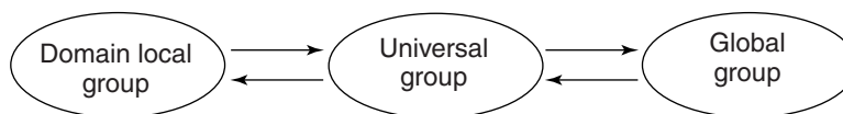
FIGURE 3.30 You can change a group scope to and from a universal group, but you can't change scope directly from a domain local group to a global group or vice versa.
