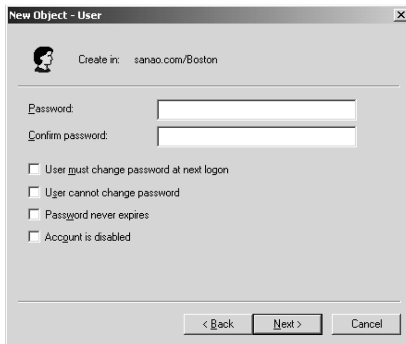
FIGURE 3.10 On the second page of the user creation wizard, you can specify a password and the way it will be used.
