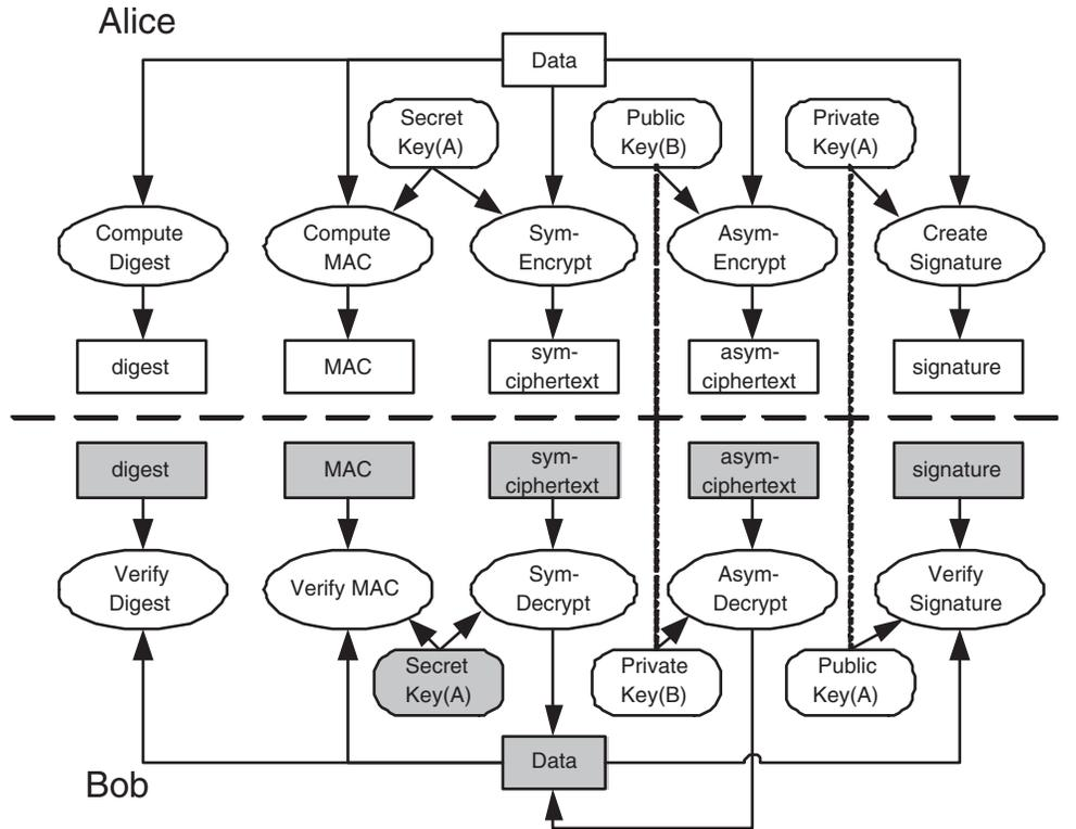
**Figure 3-3** Cryptographic operations and their uses.
