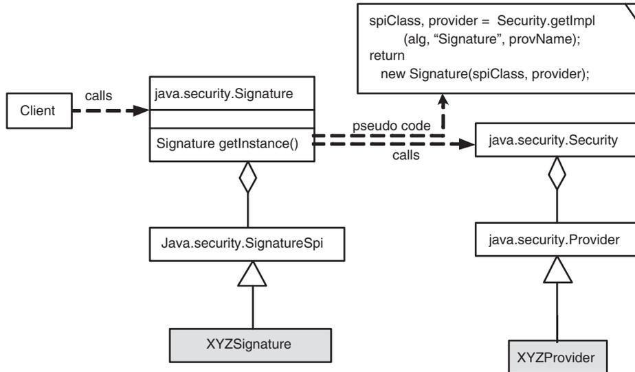
**Figure 3-1** Provider Architecture for Signature Class.
