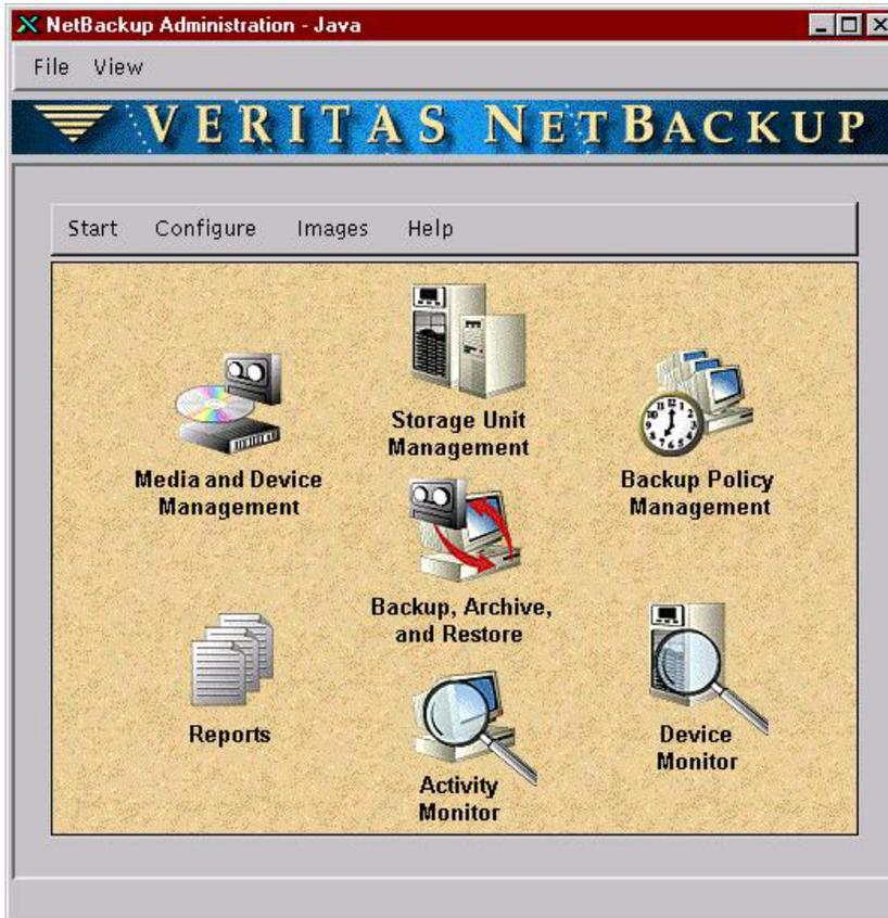
**FIGURE 1-2** The NetBackup GUI supports centralized administration of a backup and restore architecture that may include widely distributed nodes located throughout a global enterprise. The Java™ technology version of the GUI is shown.
