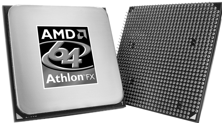
Figure 3.45 AMD Athlon 64 FX (Socket 939 version). Photo courtesy of AMD.
