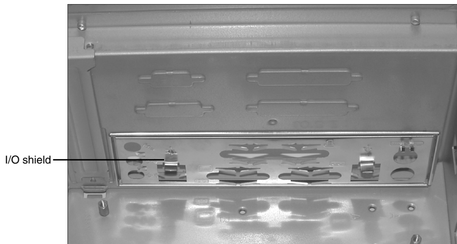
Figure 19.13 The I/O shield after being snapped into place in the chassis.
