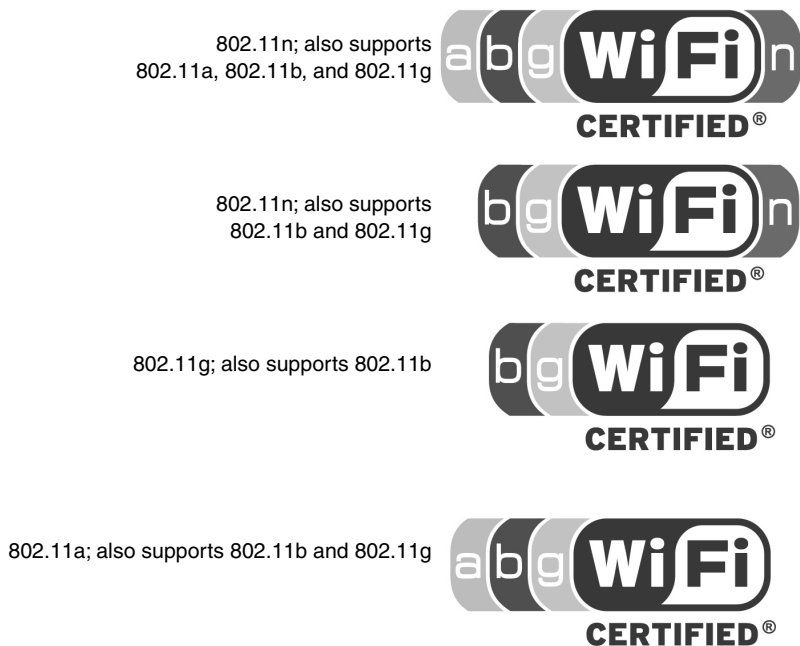
Figure 17.3 The Wi-Fi Alliance's certification labels for Wi-Fi-compliant 802.11 hardware.
