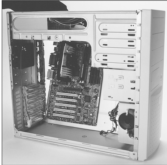
Figure 19.14 Installing a motherboard and tray into the chassis.
