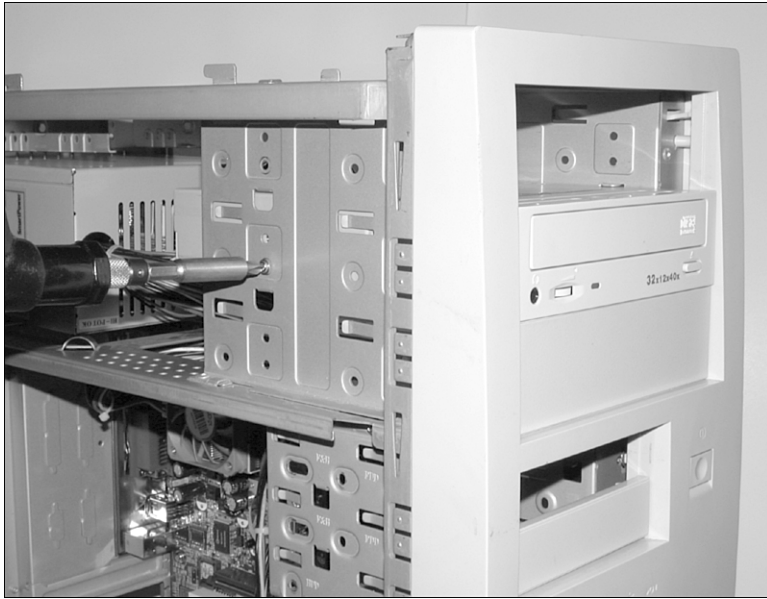
Figure 19.22 Secure the drive to the chassis using four screws.
