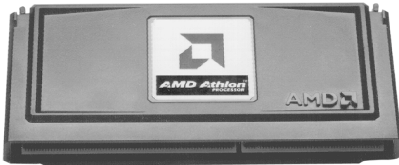
Figure 3.42 AMD Athlon processor for Slot A (cartridge form factor).
