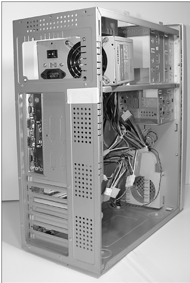
Figure 19.16 Installing the power supply into the chassis.
