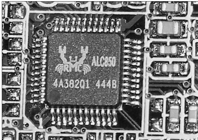
Figure 13.4 The Realtek ALC850 is a typical AC'97 2.3-compliant codec chip with surround audio support.
