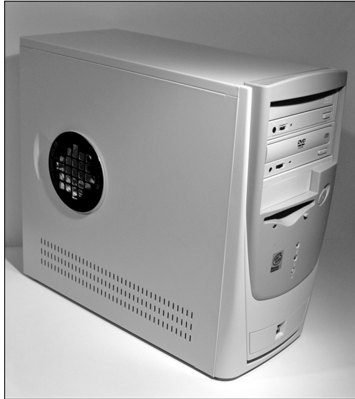
Figure 3.59 Processor duct installed.
