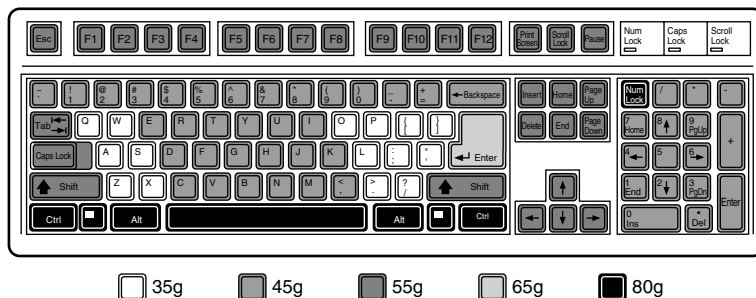
Figure 15.5 Force levels used on KeyTronicEMS keyboards with Ergo Technology.
