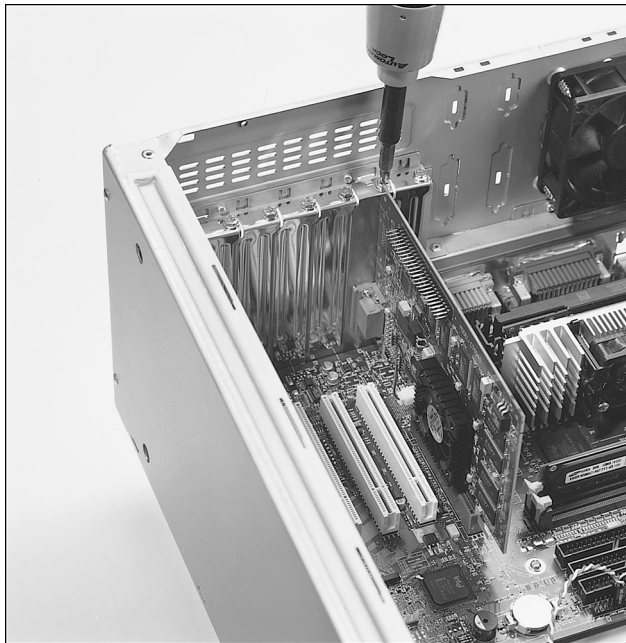
Figure 19.25 Installing the screw to retain the card.
