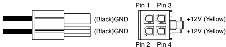
Figure 18.23 +12V 4-pin CPU power connector, side and terminal end view.
