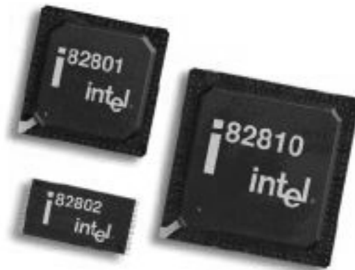
Figure 4.30 Intel 810 chipset showing the 82810 (GMCH), 82801 (ICH), and 82802 (FWH) chips. Photograph used by permission of Intel Corporation.
