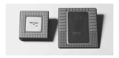
FIG. 3.2 PGA on Pentium 66 (left) and dual-pattern SPGA on Pentium Pro (right).
