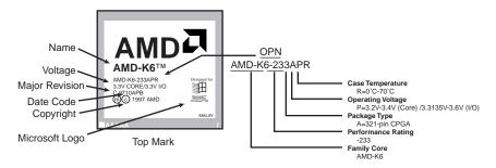
**FIG. 3.29** AMD K6 processor markings.
