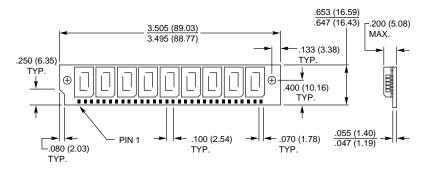
**FIG. 5.5** A typical 30-pin SIMM. The one shown here is 9-bit, although the dimensions would be the same for 8-bit as well.
