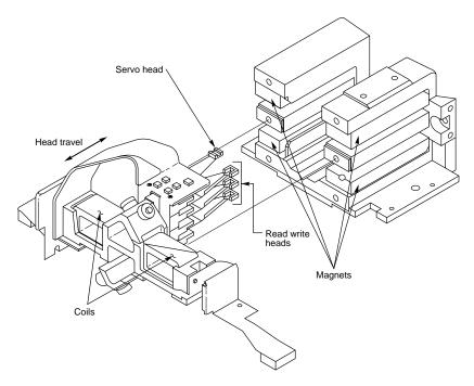
**FIG. 12.7** A linear voice coil actuator.
