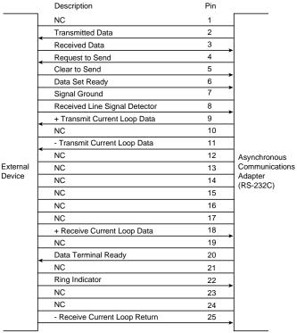
FIG. 10.2 Standard 25-pin serial-port connector specifications.
