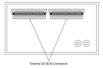
**FIG. 13.9** Older Centronics-style external CD-ROM drive SCSI connectors.
