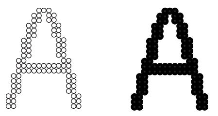
**FIG. 14.1** Because printed characters are composed of individual dots, lower resolution images can contain diagonal lines in which a jagged effect is quite obvious.
