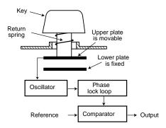
**FIG. 7.7** A capacitive keyswitch.
