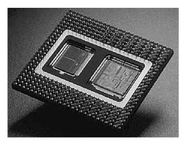
FIG. 3.23 Pentium Pro Processor with 256K L2 cache (left). Photograph used by permission of Intel Corporation.
