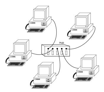
**FIG. 11.17** The star topology, linking the LAN's computers and devices to one or more central hubs, or access units.
