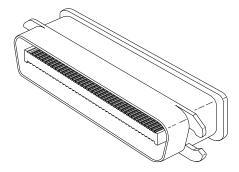
**FIG. 10.7** External SCSI device terminator.
