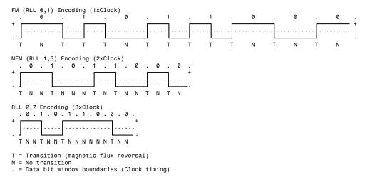
FIG. 12.2 ASCII character "X" write waveforms using FM, MFM, and RLL 2,7 encoding.
