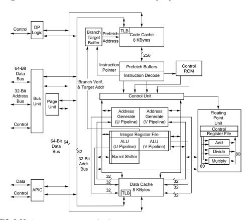
**FIG. 3.20** Pentium processor internal architecture.
