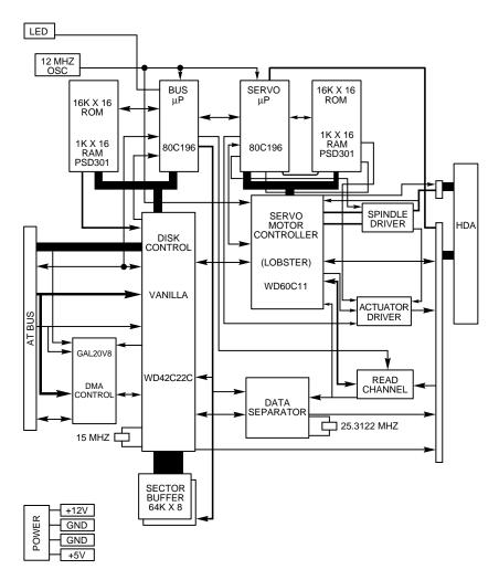
FIG. 10.9 Western Digital WD-AP4200 200M ATA-IDE drive logic-board block diagram.
