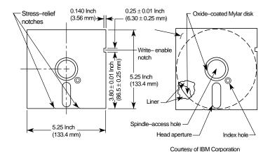
**FIG. 12.19** Construction of a 5 1/4-inch floppy disk.
