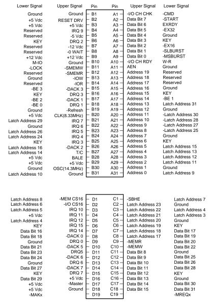
FIG. 4.18 Pinouts for the EISA bus.
