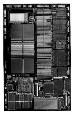
FIG. 3.19 486 Processor die. Photograph used by permission of Intel Corporation.
