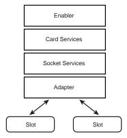
**FIG. 15.12** The Card and Socket Services enable an operating system to recognize the PC Card inserted into a slot and configure the appropriate system hardware resources for the device.
