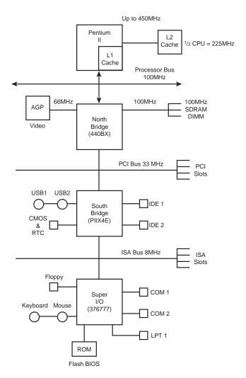
**FIG. 4.13** Typical Pentium II (P6 Class) system architecture showing the different bus levels in the system.
