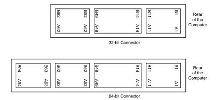
**FIG. 4.28** The universal PCI slot and card configuration.
