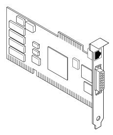
**FIG. 11.9** The network interface adapter sends and receives messages to and from all the computers on the LAN.
