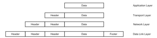
**FIG. 11.7** Each protocol in a computer's networking stack encapsulates the data it receives from the layer above by adding its own header.
