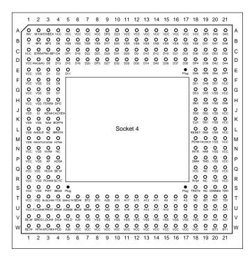
**FIG. 3.11** 273-pin Intel Socket 4 configuration.
