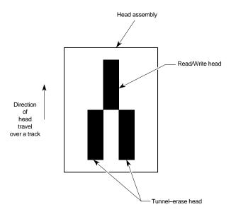
**FIG. 12.16** Composite construction of a typical floppy disk drive head.
