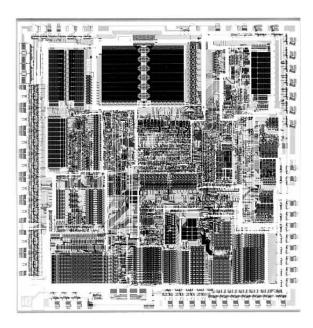
FIG. 3.17 286 Processor die. Photograph used by permission of Intel Corporation.
