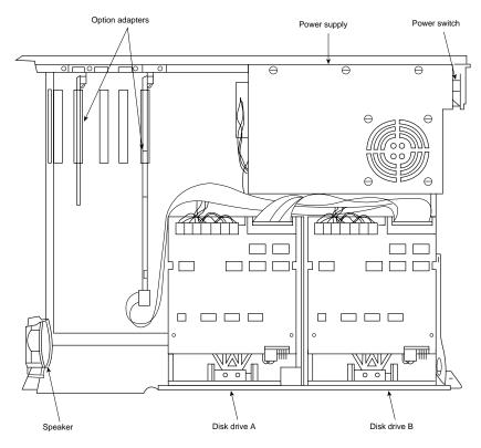
**FIG. 20.1** The IBM PC interior view.
