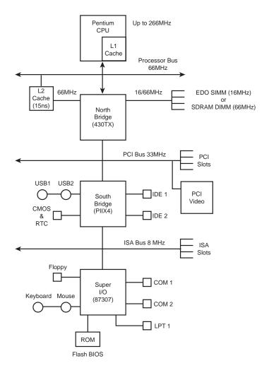
FIG. 5.4 System Architecture, Pentium MMX system with an Intel 430TX chipset.
