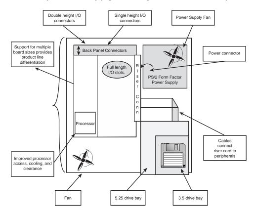
**FIG. 4.7** NLX system chassis layout and features.
