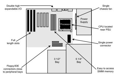
FIG. 4.4 ATX system chassis layout and features.
