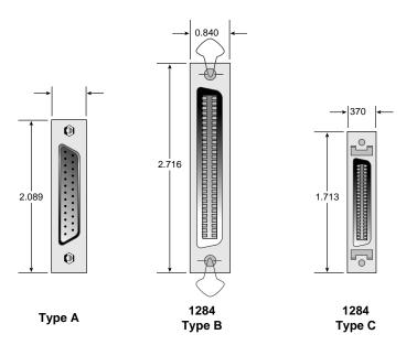
**FIG. 10.3** The three different IEEE 1284 connectors.
