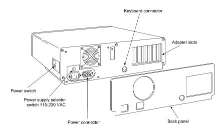
**FIG. 20.10** The IBM AT rear panel.
