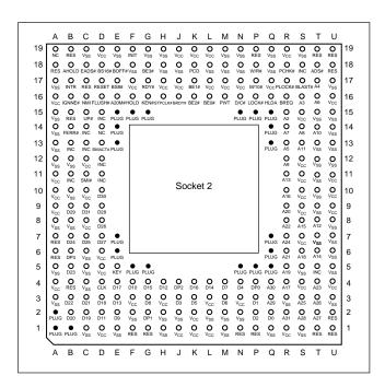
FIG. 3.8 238-pin Intel Socket 2 configuration.
