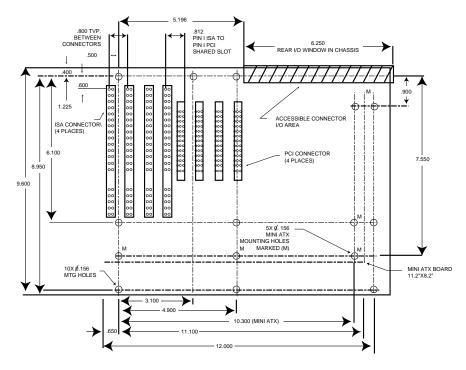
FIG. 16.2 ATX motherboard form factor.
