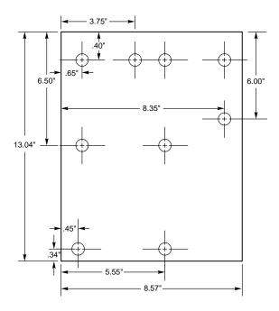
**FIG. 4.1** Baby-AT motherboard form factor.
