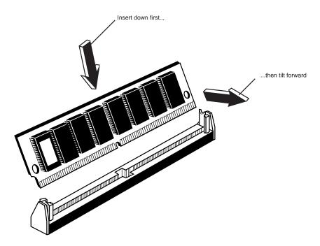
**FIG. 5.10** The notch on this SIMM is shown on the left end. Insert the SIMM at an angle and then tilt it forward until the locking clips snap into place.
