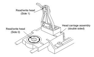
**FIG. 12.15** A double-sided drive head assembly.
