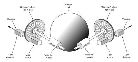
**FIG. 7.16** Typical opto-mechanical mouse mechanism.
