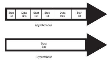
**FIG. 11.1** Asynchronous modems frame each byte of data with a start bit and a stop bit, while synchronous communications use an uninterrupted stream of data.
