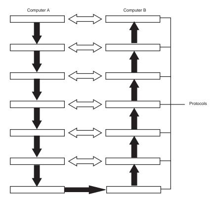
**FIG. 11.8** Protocols in the networking stack communicate indirectly with their equivalent protocols in other computers.
