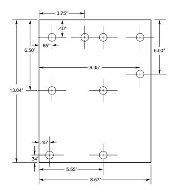
FIG. 16.1 Baby-AT motherboard form factor.
