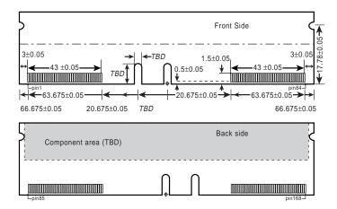
FIG. 5.3 168-pin RIMM module.
