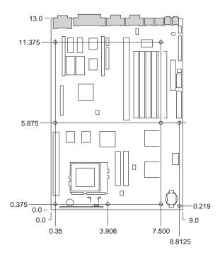
FIG. 4.2 LPX motherboard dimension.
