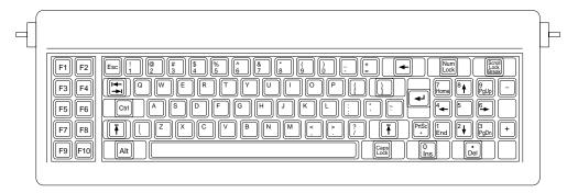
**FIG. 7.1** PC and XT 83-key keyboard layout.
