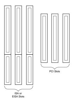
**FIG. 4.25** Possible configuration of PCI slots in relation to ISA or EISA slots.
