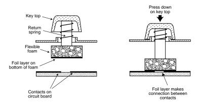
**FIG. 7.6** Typical foam element mechanical keyswitch.
