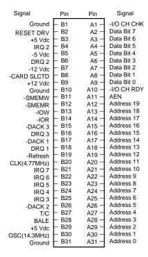
FIG. 4.14 Pinouts for the 8-bit ISA bus.
