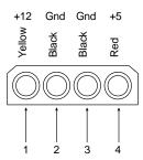
**FIG. 12.17** A disk drive female power supply cable connector.
