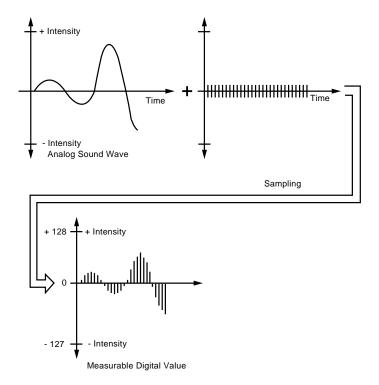
FIG. 9.3 Sampling turns a changing sound wave into measurable digital values.
