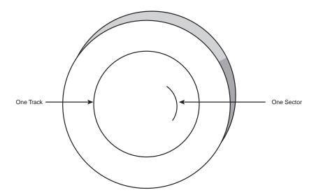
**FIG. 12.3** The tracks and sectors of a hard disk drive.
