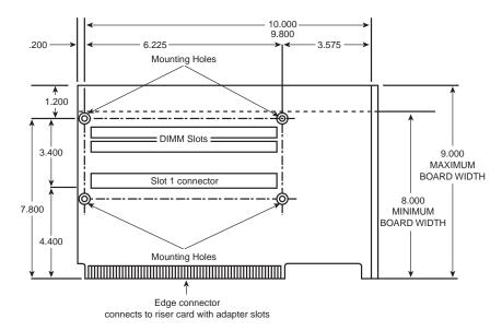
**FIG. 4.8** NLX form factor. This shows a 10-inch long NLX board. The NLX specification also allows 11.2-inch and 13.6-inch long versions.
