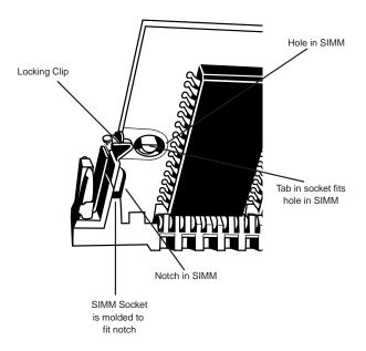
**FIG. 5.11** This closeup shows the backside of a SIMM inserted in the SIMM socket with the notch aligned, the locking clip locked, and the hole in the SIMM aligned with the tab that sticks out from the socket.
