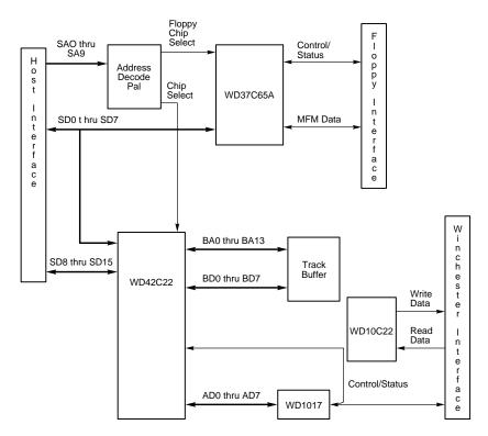
FIG. 10.11 Western Digital WD1006V-MM1 ST-506/412 Disk Controller block diagram.
