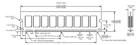
**FIG. 5.7** A typical 168-pin DIMM. The one shown here is 72-bit, although the dimensions would be the same for 64-bit as well.
