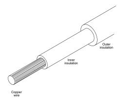
FIG. 11.14 Coaxial cable.
