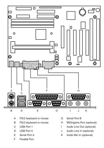
**FIG. 4.6** Typical ATX motherboard rear panel connectors.
