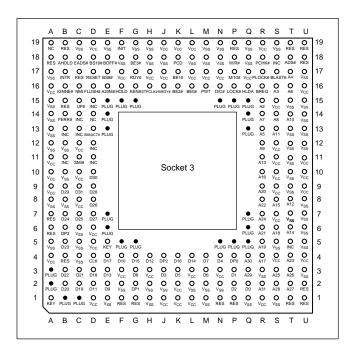
**FIG. 3.10** 237-pin Intel Socket 3 configuration.
