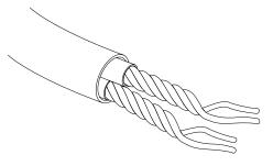
**FIG. 11.12** A shielded twisted-pair cable.
