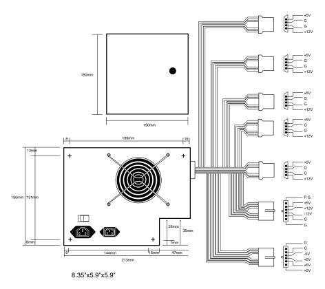
**FIG. 6.3** AT/Tower form factor power supply.
