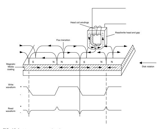
FIG. 12.1 Magnetic write and read processes.
