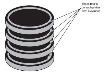
FIG. 12.4 A hard disk cylinder.
