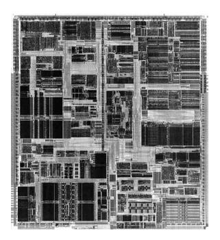
FIG. 3.25 Pentium II Processor die. Photograph used by permission of Intel Corporation.
