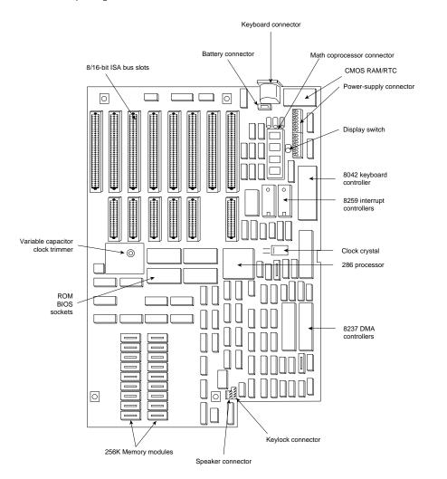
**FIG. 20.12** The IBM AT Type 2 motherboard.
