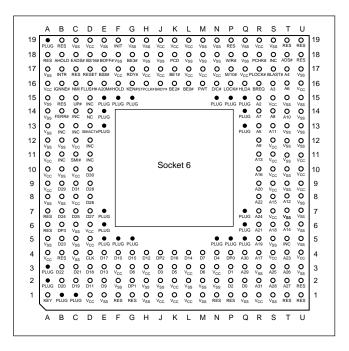
**FIG. 3.13** 235-pin Intel Socket 6 configuration.
