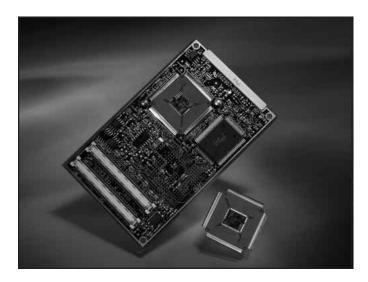
**FIG. 15.8** Mobile Pentium Processors in mobile module or raw Tape Carrier Package form. *Photograph used by permission of Intel Corporation.*
