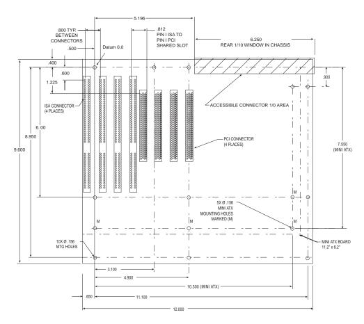
**FIG. 4.5** ATX specification version 2.01.
