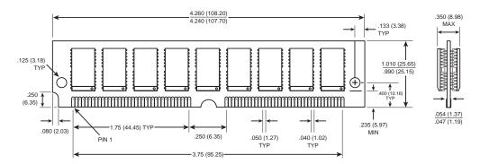
**FIG. 5.6** A typical 72-pin SIMM. The one shown here is 36-bit, although the dimensions would be the same for 32-bit as well.
