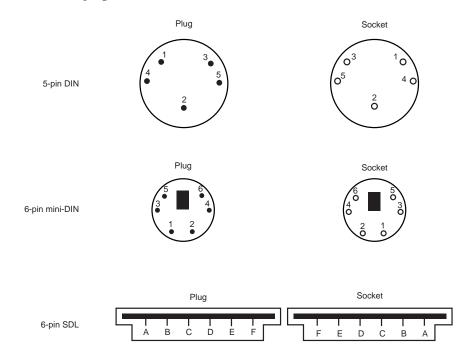
FIG. 7.14 Keyboard and mouse connectors.
