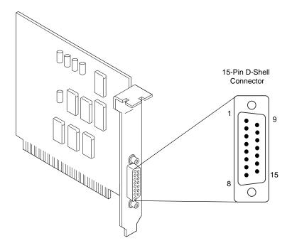
**FIG. 7.19** Typical game adapter and 15-pin connector.
