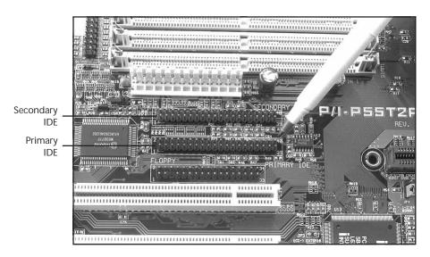
FIG. 13.8 An embedded EIDE interface with a primary and secondary IDE connection.
