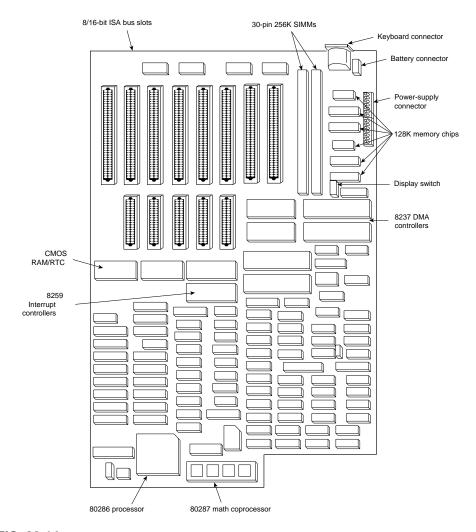
FIG. 20.14 The IBM XT-286 motherboard.
