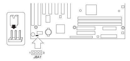
**FIG. 4.9** Typical Intel motherboard BIOS recovery jumper.
