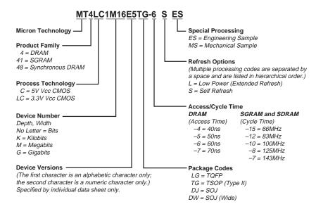
FIG. 5.9 Typical SIMM part numbers for Micron (Crucial Technology) SIMMs.
