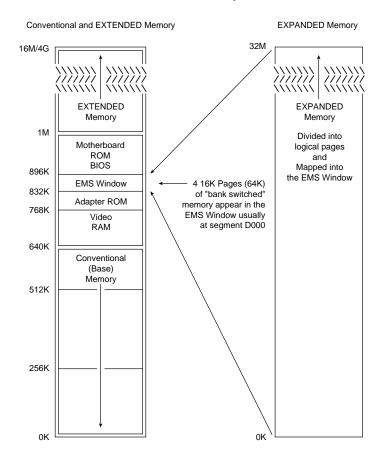
**FIG. 5.22** Conventional, extended, and expanded memory.
