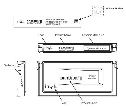
FIG. 3.28 Pentium II Single Edge Contact Cartridge.
