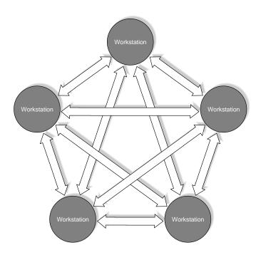
**FIG. 11.5** The logical architecture of a typical peer-to-peer network.
