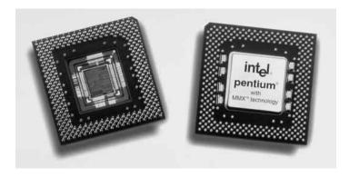
**FIG. 3.1** An Intel Pentium MMX chip shown from the top and bottom (exposing the die). *Photograph used by permission of Intel Corporation.*
