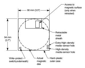
**FIG. 12.20** Construction of a 3 1/2-inch floppy disk.
