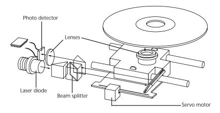
**FIG. 13.1** Typical components inside a CD-ROM drive.
