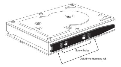
**FIG. 12.12** A typical hard disk with mounting rails.
