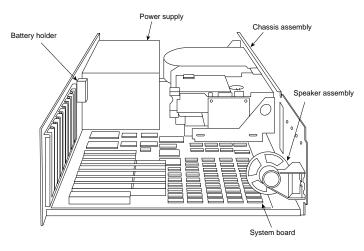
FIG. 20.13 The IBM XT-286 interior.
