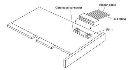
**FIG. 13.10** Connecting a ribbon cable to a SCSI adapter.
