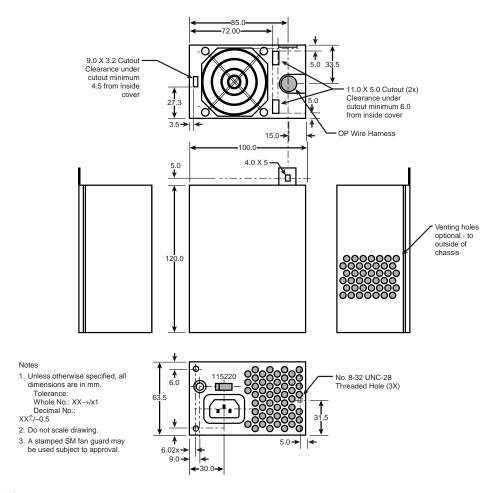
**FIG. 6.7** SFX form factor power supply.
