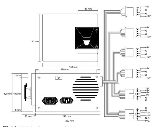
**FIG. 6.1** PC/XT form factor power supply.
