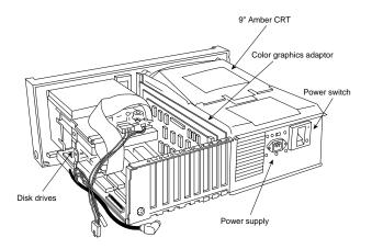
FIG. 20.8 The IBM Portable PC interior.
