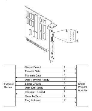
FIG. 10.1 AT-style 9-pin serial-port connector specifications.
