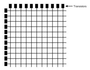
**FIG. 15.1** Dual scan LCD displays use a combination of two transistors on intersecting axes to control the color of each pixel.
