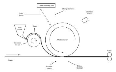
**FIG. 14.4** A laser printer's print engine largely revolves around a photoreceptor drum that receives the document image from the laser and applies it to the page as it slowly rotates.
