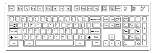
FIG. 7.3 101-key Enhanced keyboard layout.
