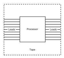
**FIG. 15.4** A processor that is mounted using the tape carrier package is attached to a piece of copper-laminated film that replaces the pins used in standard desktop processors.
