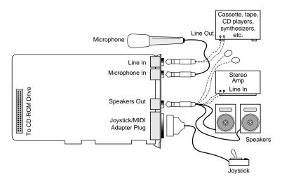
FIG. 9.5 The basic input and output connectors that most audio adapters have in common.
