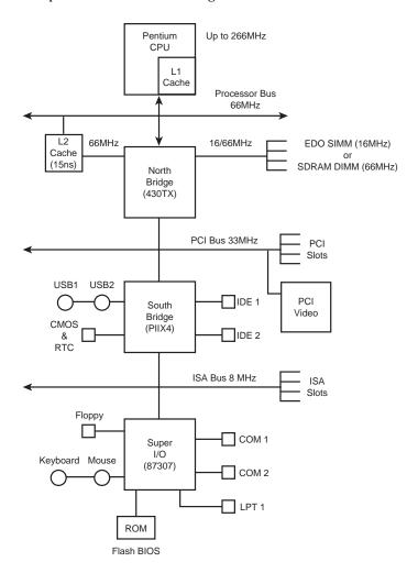
**FIG. 4.12** Typical Pentium (P5 Class) system architecture showing the different bus levels in the system.
