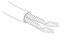
**FIG. 11.11** An unshielded twisted-pair cable.
