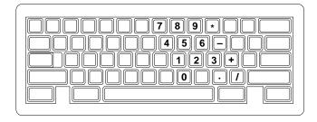
**FIG. 7.5** Most portable systems today embed the numeric keypad into an oddly shaped block of keys on the alphabetical part of the keyboard.
