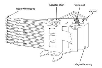
**FIG. 12.6** Read/write heads and rotary voice coil actuator assembly.
