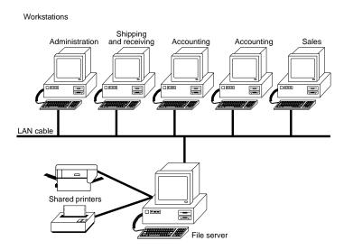
**FIG. 11.4** The components of a client/server LAN.
