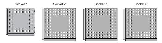
FIG. 3.5 486 Processor Sockets.
