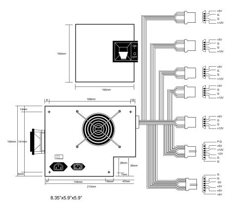
**FIG. 6.2** AT/Desktop form factor power supply.
