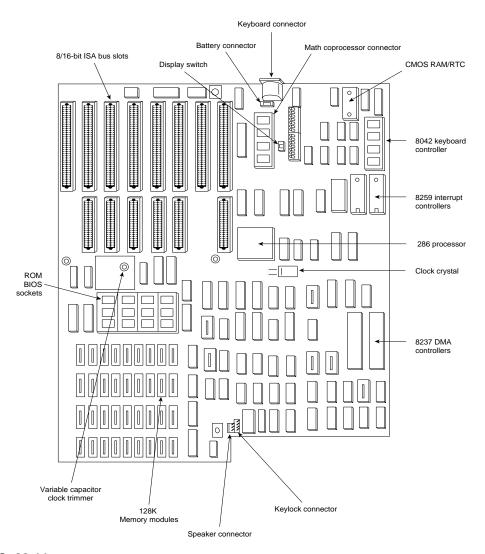
**FIG. 20.11** The IBM AT Type 1 motherboard.
