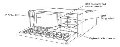
FIG. 20.7 The IBM Portable PC.
