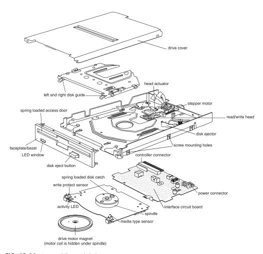
FIG. 12.14 A typical floppy disk drive.
