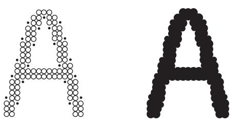
**FIG. 14.2** Resolution Enhancement Technology mixes dots of different sizes to lessen the jagged effect seen in low resolution images.
