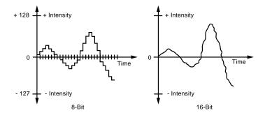
FIG. 9.4 16-bit resolution allows more accurate sound reproduction than 8-bit resolution.
