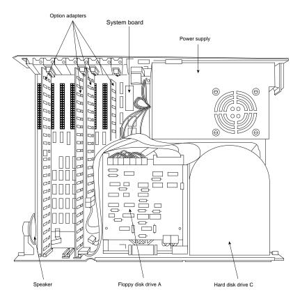
**FIG. 20.5** The IBM PC XT interior.
