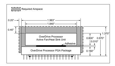
FIG. 3.9 The physical dimensions of the Intel Pentium OverDrive processor and active heat sink.
