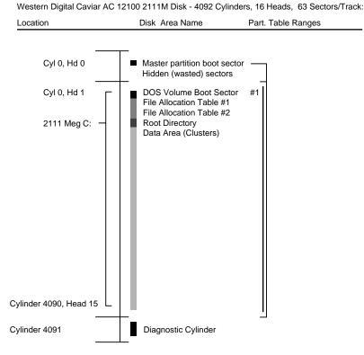
FIG. 19.1 DOS disk management structures on a Western Digital Caviar AC12100.
