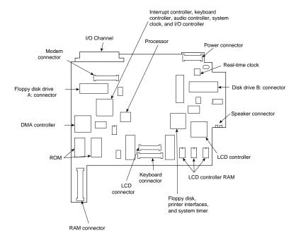
**FIG. 20.4** The PC Convertible motherboard.
