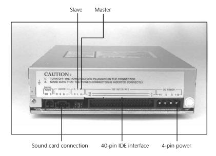
**FIG. 13.7** The rear connection interfaces of a typical IDE internal CD-ROM drive.
