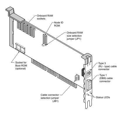
FIG. 11.10 The Thomas-Conrad 16/4 Token Ring adapter (with DB9 and RJ45 connectors).
