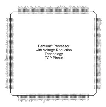
FIG. 15.7 Intel Mobile Pentium Tape Carrier Package Pinout.
