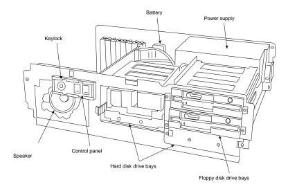
**FIG. 20.9** The IBM AT unit interior.
