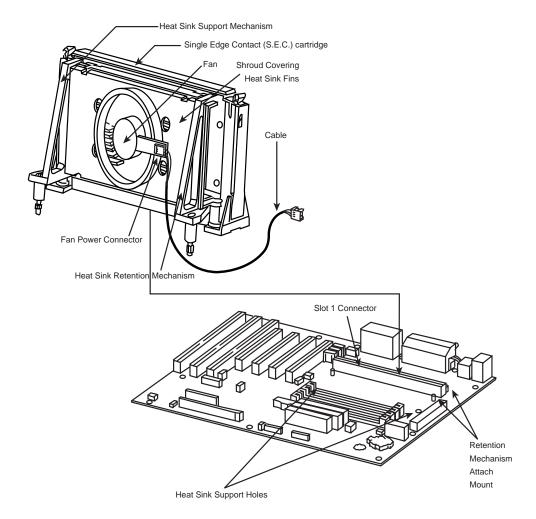
FIG. 3.27 Pentium II Processor and Heat Sink Assembly.
