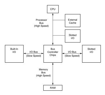
FIG. 4.21 How a local bus works.
