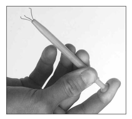
FIG. 17.7 The parts grabber has three small metal prongs that can be extended to grab a part.
