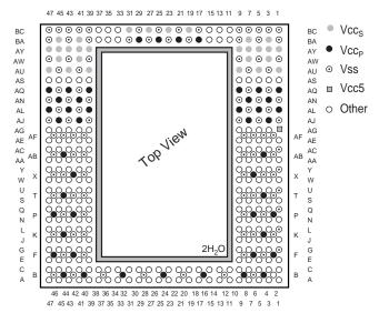
**FIG. 3.15** Socket 8 (Pentium Pro) Pinout showing power pin locations.
