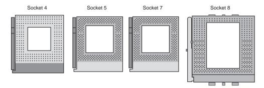
FIG. 3.6 Pentium and Pentium Pro Processor Sockets.
