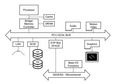
FIG. 4.24 Conceptual diagram of the PCI bus.
