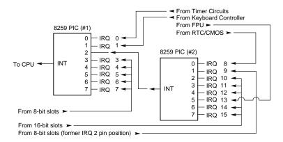
FIG. 4.29 Interrupt controller cascade wiring.
