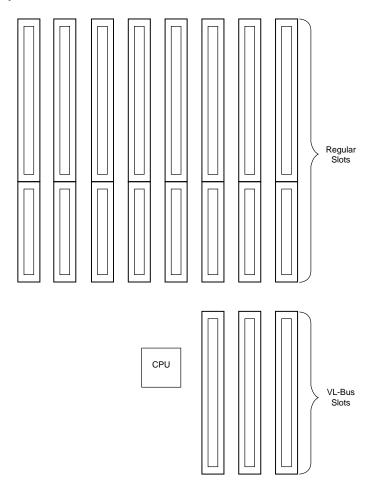
**FIG. 4.22** An example of VL-Bus slots in an ISA system.
