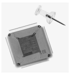
**FIG. 15.5** Pentium MMX Processor in TCP Mobile Package. *Photograph used by permission of Intel Corporation.*
