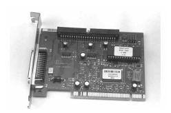
FIG. 10.12 An Adaptec AHA-2940AU SCSI host adapter.
