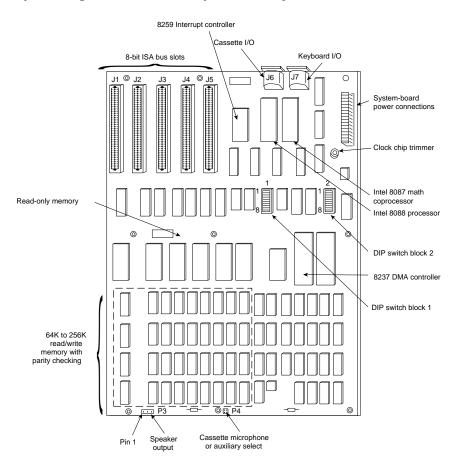
FIG. 20.3 The IBM PC motherboard.
