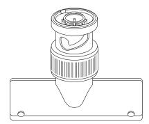
FIG. 11.13 An Ethernet coaxial cable T-connector.
