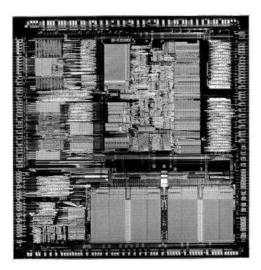
FIG. 3.18 386 Processor die. Photograph used by permission of Intel Corporation.
