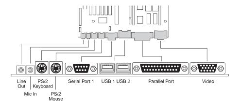
FIG. 4.3 LPX motherboard back panel connectors.
