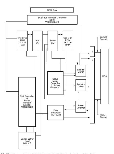
FIG. 10.10 Western Digital WD-SP4200 200M SCSI drive logic-board block diagram.
