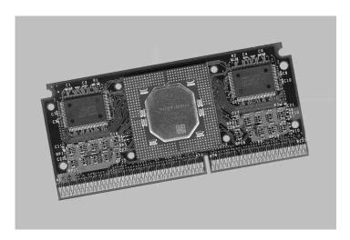
**FIG. 3.26** Pentium II Processor Board (inside SEC cartridge). *Photograph used by permission of Intel Corporation.*
