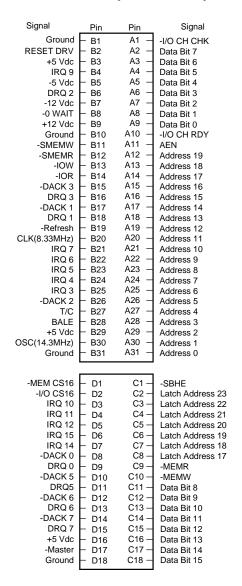
FIG. 4.16 Pinouts for the 16-bit ISA bus.
