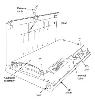
**FIG. 7.15** Typical keyboard components.
