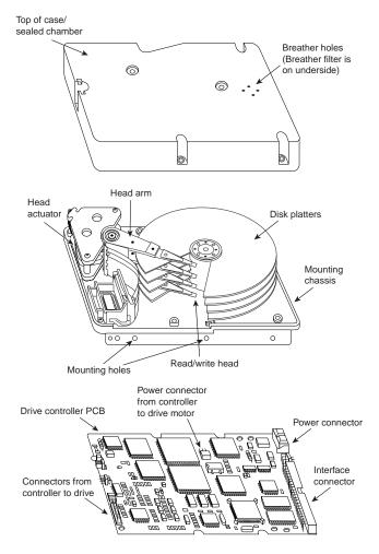
FIG. 12.5 Hard disk drive components.
