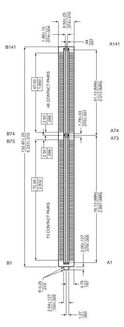
**FIG. 3.16** Slot 1 connector dimensions and pin layout.
