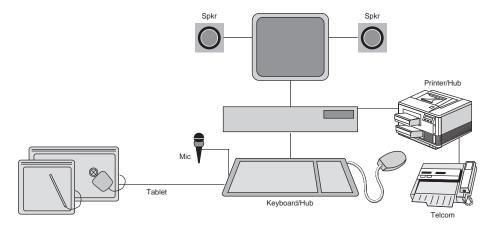
**FIG. 10.4** A PC can use multiple USB hubs to support a variety of different peripherals connected to whichever hub is most convenient.
