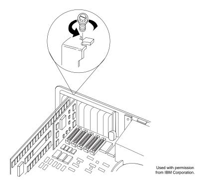
**FIG. 16.5** Insert the adapter into a slot and screw it in place.
