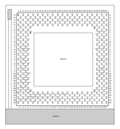
**FIG. 3.12** 320-pin Intel Socket 5 configuration.
