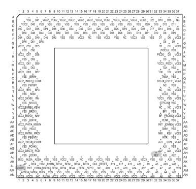
**FIG. 3.14** Socket 7 (Pentium) Pinout—top view.
