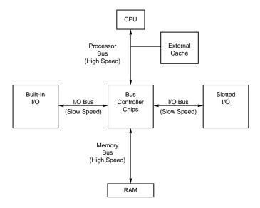
FIG. 4.20 Bus layout in a traditional PC.
