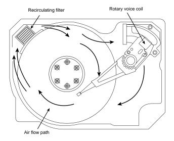
**FIG. 12.10** Air circulation in a hard disk.
