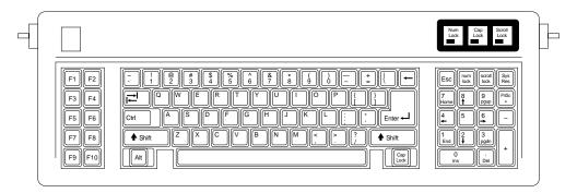
FIG. 7.2 AT 84-key keyboard layout.
