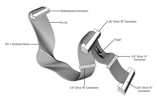
**FIG. 12.18** Standard five-connector floppy interface cable.
