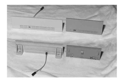
**FIG. 12.11** Typical 5 1/4- and 3 1/2-inch hard drives bezel shown from the front (as seen on the outside of the PC case) (top) and from the back (bottom) (the inside mounting and LED wiring).
