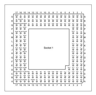
FIG. 3.7 Intel Socket 1 pinout.
