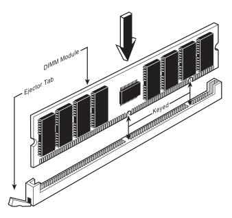
**FIG. 5.12** DIMMs keys match the protrusions in the DIMM sockets.
