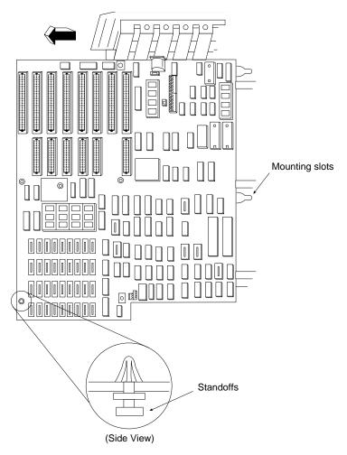
**FIG. 16.3** Insert standoffs into their mounting slots.
