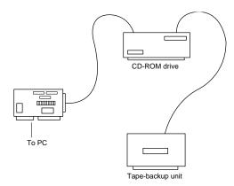
**FIG. 13.12** A SCSI chain of devices on one adapter card.
