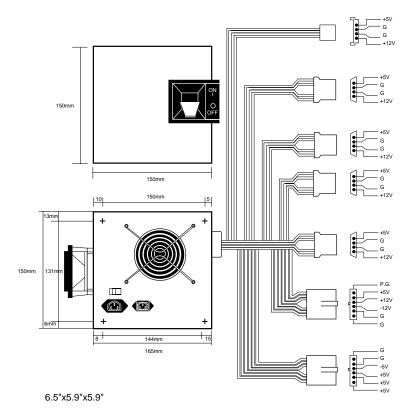
**FIG. 6.4** Baby AT form factor power supply.
