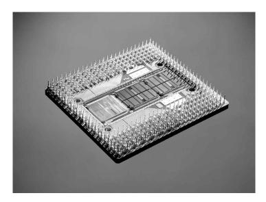
**FIG. 3.24** Pentium Pro Processor with 1M L2 cache (center and right). *Photograph used by permission of Intel Corporation.*
