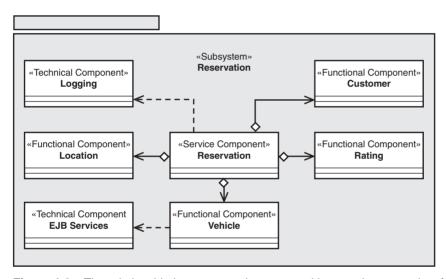
**Figure 4-6** The relationship between a subsystem and its constituent service, functional, and technical components
