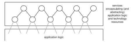
**Figure 3.14**Application logic created with proprietary technology can be abstracted through a dedicated service layer.
