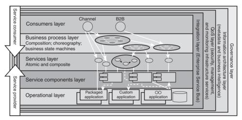
Figure 4-1 Logical view of SOA Reference Architecture
