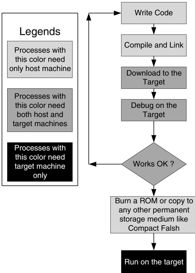
**Figure 8-1** Flow chart of cross-platform development.
