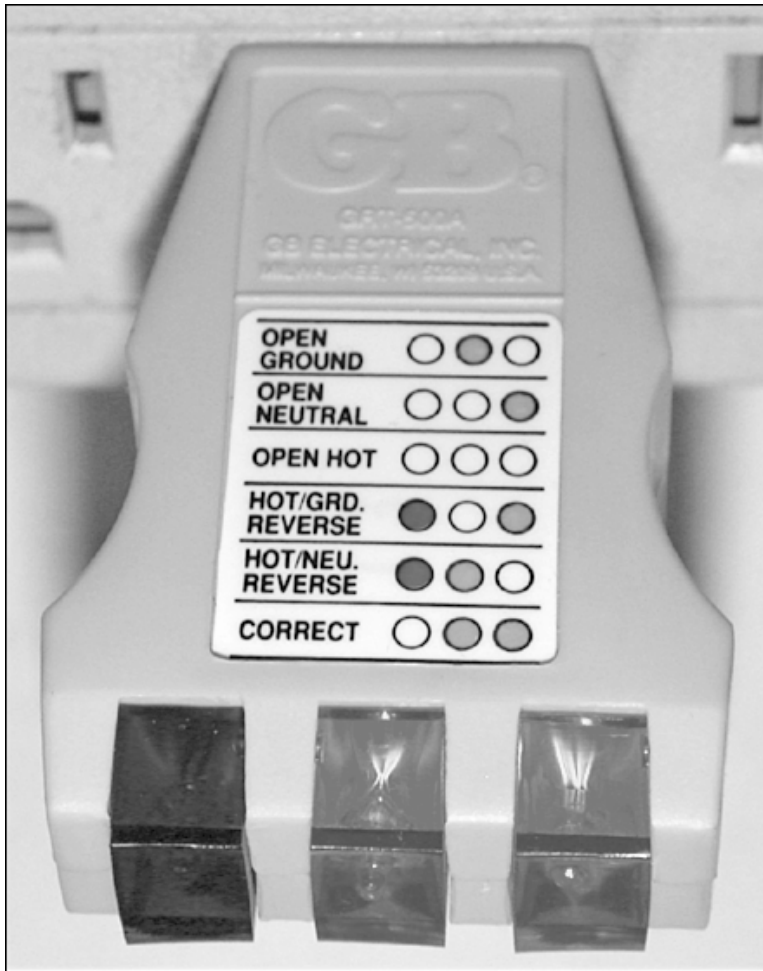
Figure 5-12 An outlet tester like this one can find wiring problems quickly. This outlet is wired correctly.
