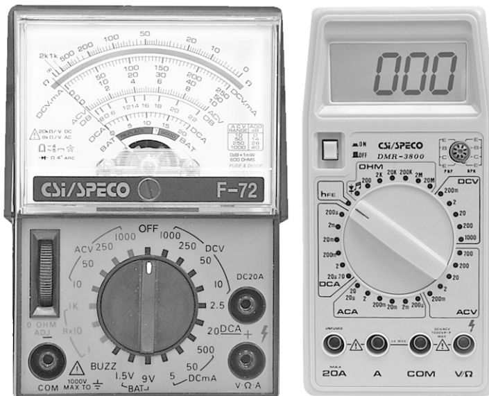
Figure 5-9 Typical analog (left) and digital (right) multimeters. Photos courtesy of Colacino Electric Supply ( www.colacinoelectric.com/ ).
