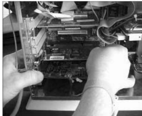
Figure 1-10 Installing an Ethernet NIC
