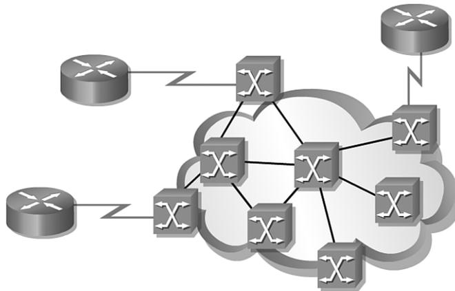
The Frame Relay WAN is mesh of interconnected switches.
