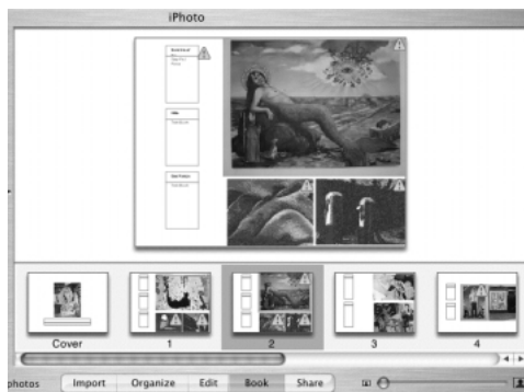
Figure 4.10 When a page design calls for a photo to be printed higher than its resolution will allow (for good quality), iPhoto places a warning icon next to the offending image (all three on the page that's showing above).
