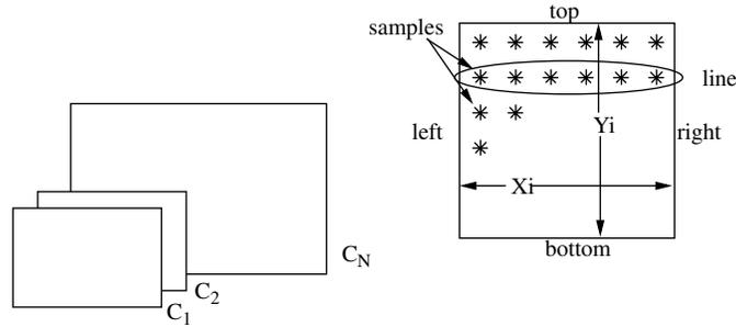
**Figure 7-4** Uncompressed digital image as per [Org93].
