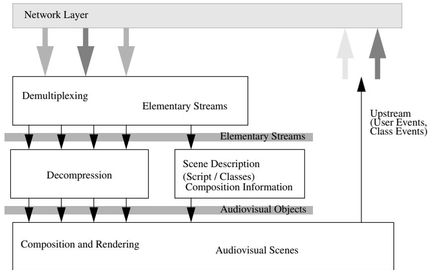
**Figure 7-24** Important components of an MPEG-4 terminal.
