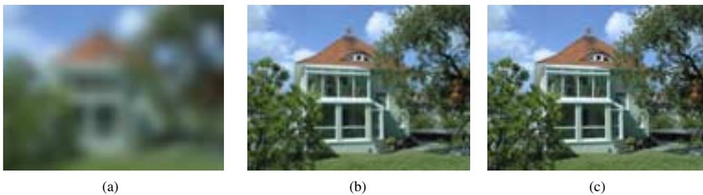
**Figure 7-16** Progressive picture presentation: (a) first phase, very unsharp image; (b) second phase, unsharp image; (c) third phase, sharp image.
