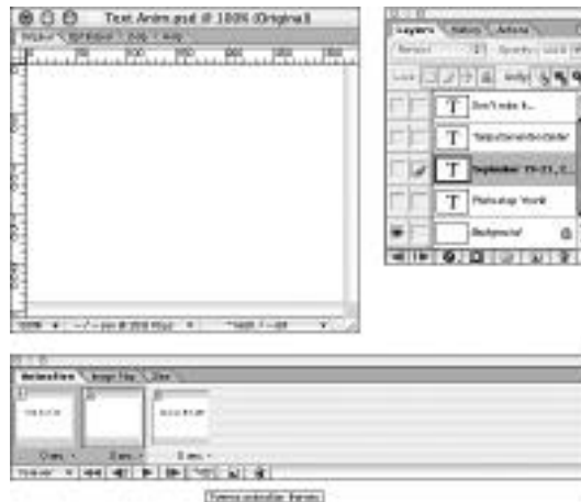
Figure 26 Select the first two frames in the Animation palette and click the Tweens Animation Frames button to select how many frames you want to add between the selected frames.
