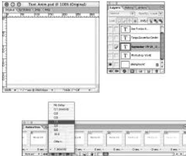
Figure 27 Adjust the timing of the text keyframes with 100% opacity so that the animation pauses briefly, giving viewers time to read the text between fades.
