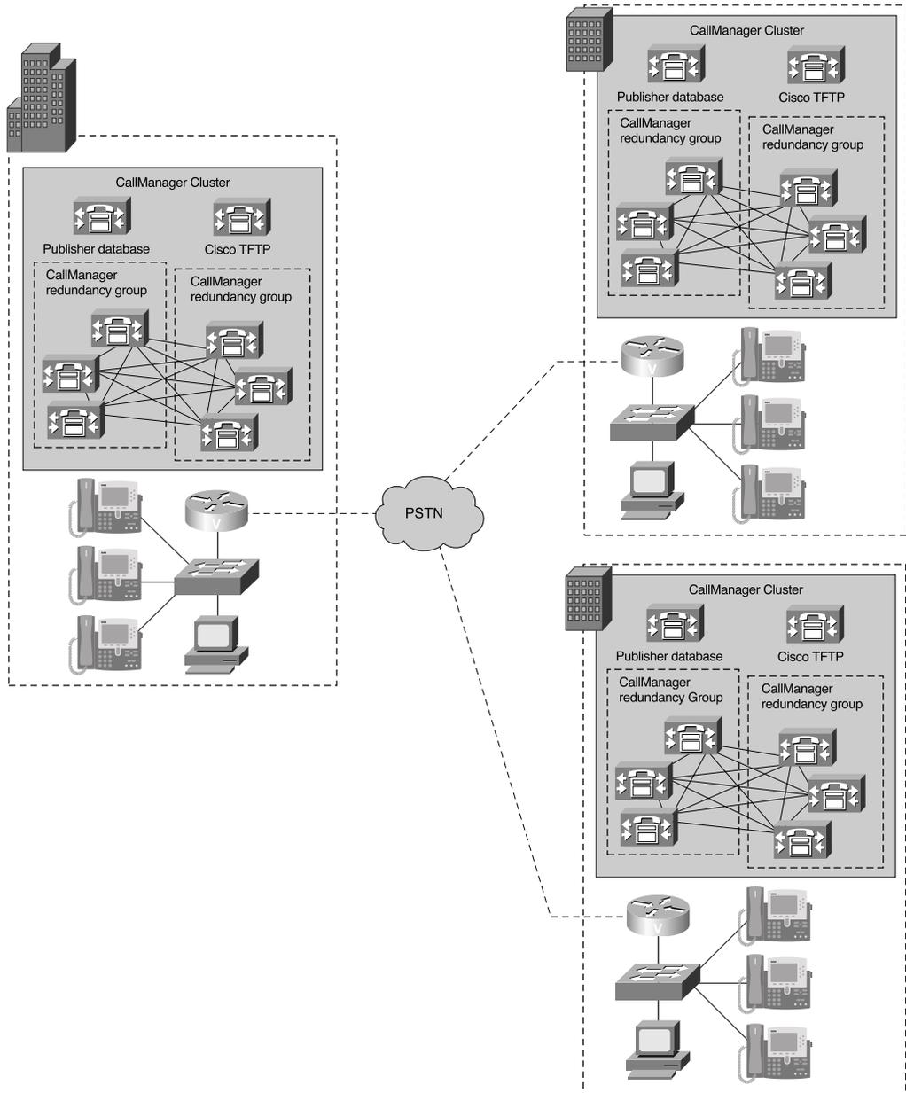
**Figure 1-19** Multiple-Site IP WAN Model with Distributed Call Processing
