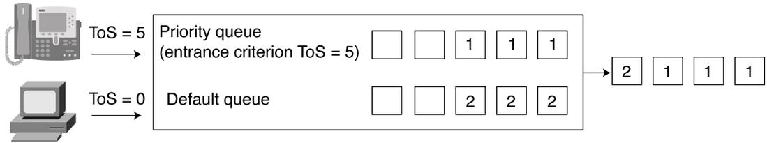
Figure 1-22 depicts two devices that send information through a network router. The Cisco IP Phone 7960 categorizes its traffic with **type of service 5**, while the PC categorizes its traffic with **type of service 0**. The router reads packets from both devices from the network and places them in queues based on the **type of service** field. Packets classified with **type of service 5** go on a priority queue, while other packets go on the default queue.
