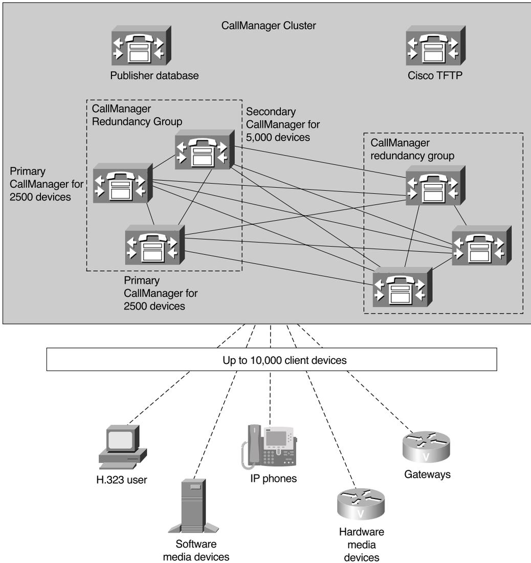
Figure 1-16 Deployment Model for More than 10,000 Users
