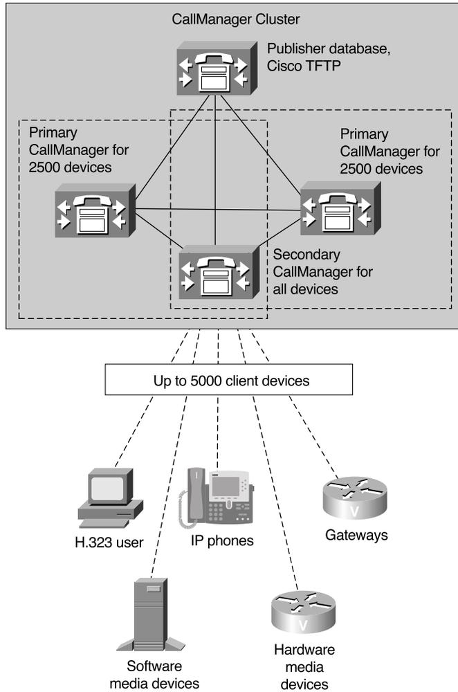
Figure 1-15 Deployment Model for 5000 to 10,000 Users
