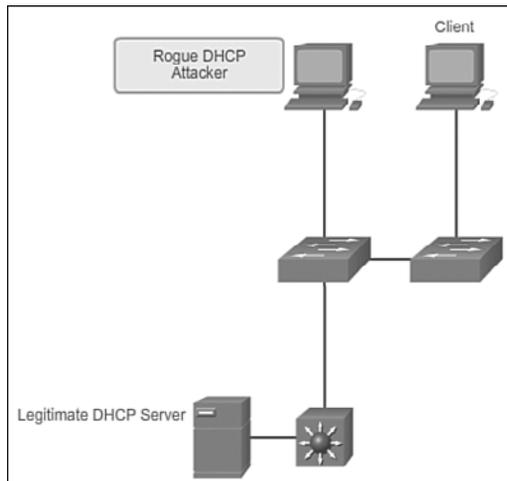
**Figure 2-21** DHCP Spoofing and Starvation Attack
