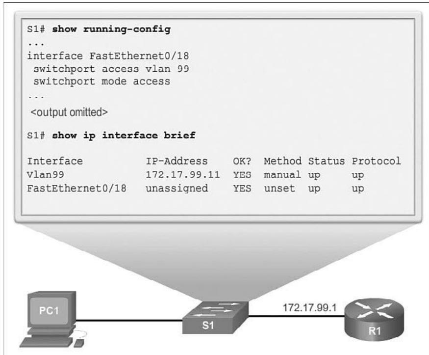
**Figure 2-6** Verifying the Switch Management Interface Configuration
