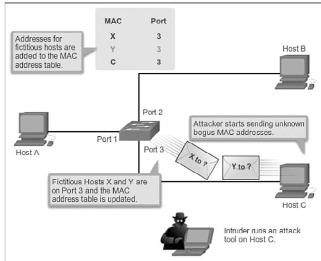
**Figure 2-19** MAC Address Flooding Attack - Attacker Launches Attack
