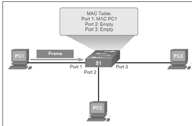
**Figure 1-14** Building a MAC Address Table: S1 Adds MAC Address Heard Through Port 1
