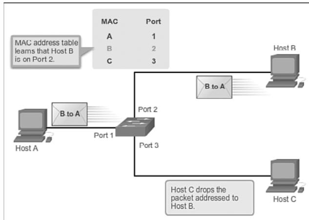
**Figure 2-17** MAC Address Flooding - Switch Records MAC Address
