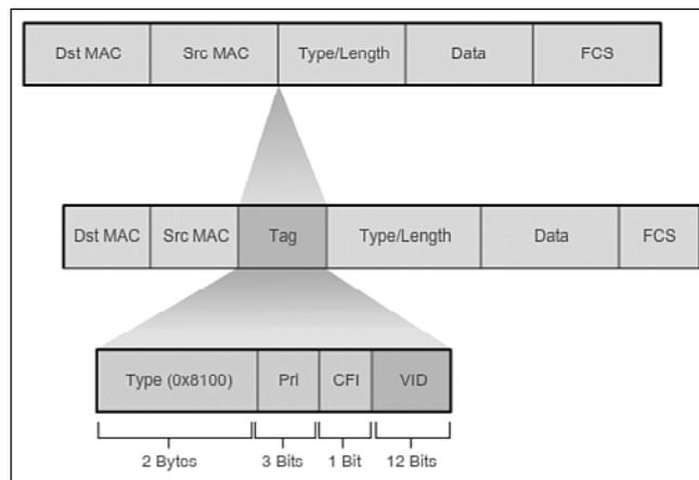
**Figure 3-9** Fields in an Ethernet 802.1Q Frame
