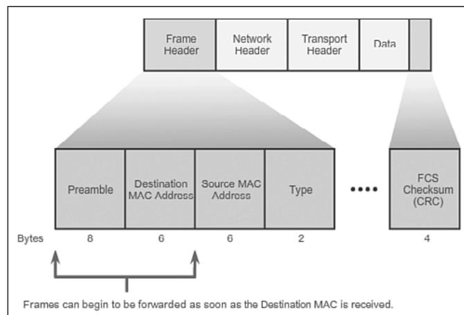
**Figure 1-20** Cut-Through Switching
