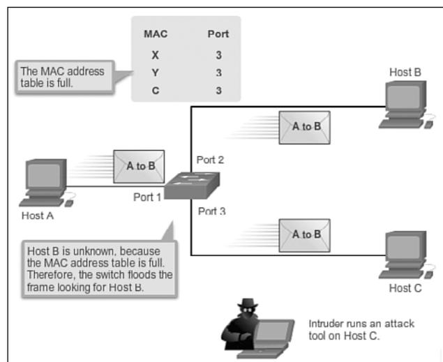
**Figure 2-20** MAC Address Flooding Attack - Attacker Sees Broadcasts
