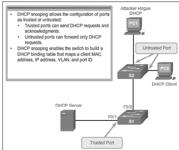
**Figure 2-24** DHCP Snooping Operation
