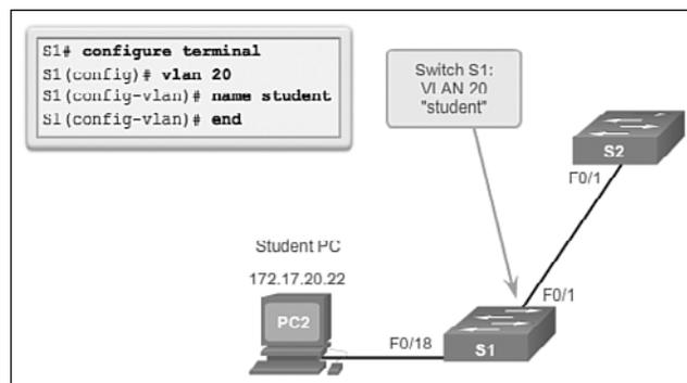
**Figure 3-14** Sample VLAN Configuration**Interactive Graphic****Activity 3.2.1.2: VLAN Creation and Verification**
