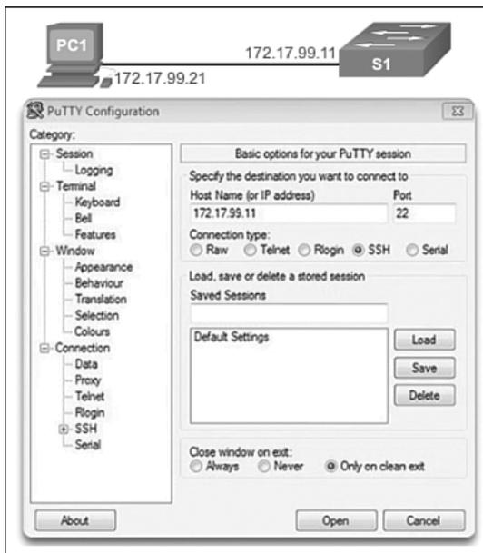
**Figure 2-13** Configure PuTTY with SSH Client Connection Parameters
