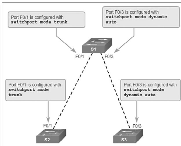
**Figure 3-20** Initial DTP Configuration
