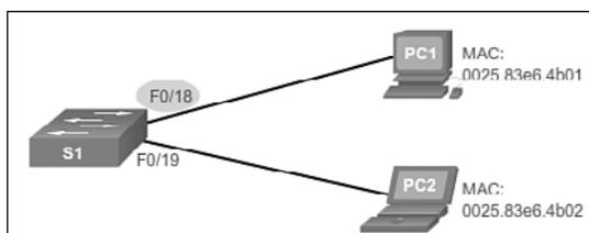
**Figure 2-26** Port Security Configuration Topology
