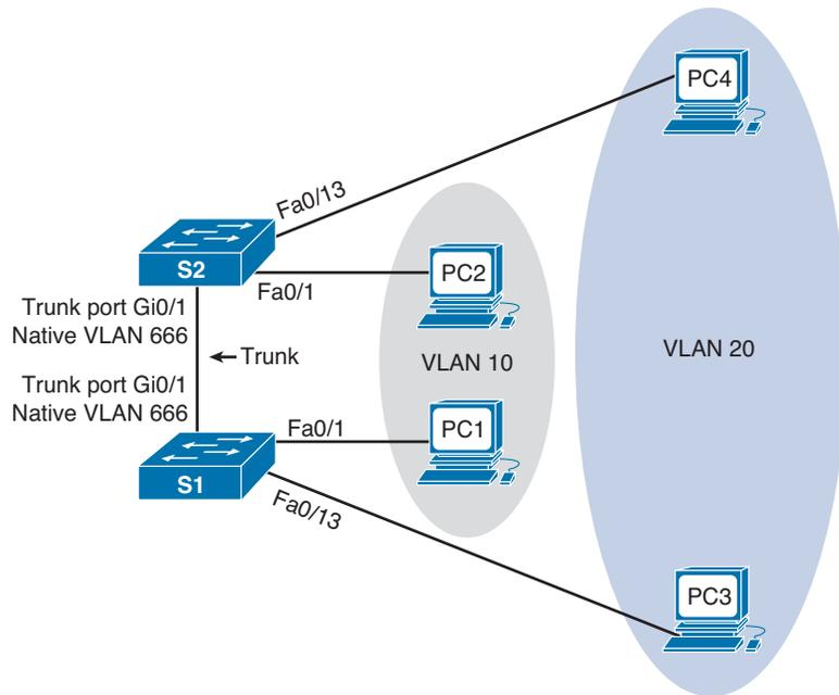
Traffic from VLANs 10 and 20 cross the trunk. A tag is added with the VLAN number before the data leaves the switch port. An unused VLAN number is configured as the native VLAN.
