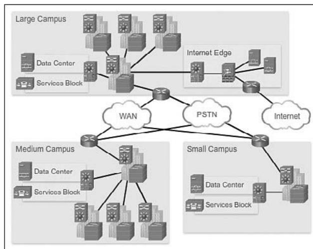
**Figure 1-9** Three-Tier Design in Borderless Switched Networks
