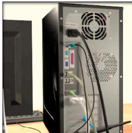
Figure 3-9 All External Cables Plugged into the Back
