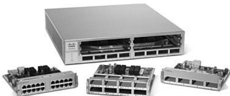
The Catalyst 4900 series switches support advanced QoS features, making them ideal candidates for the back-end IP telephony hardware. Catalyst 4900 series switches do not support the StackWise feature of the Catalyst 3750 series, nor do they support PoE.
