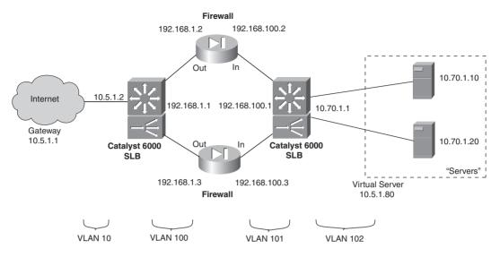
Figure 10-4 Network Diagram for the Firewall Load-Balancing Example
