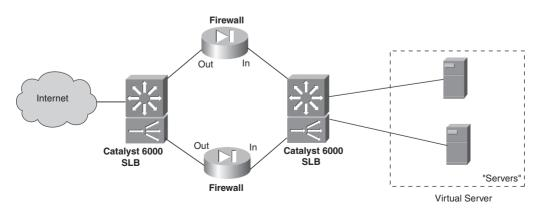
Figure 10-3 Firewall Load-Balancing Concept
