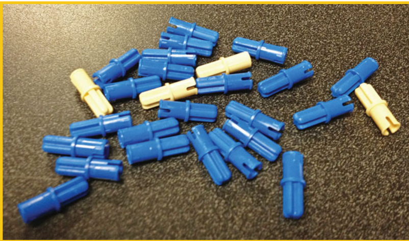
FIGURE 1.9 These pegs allow you to join two elements, one with a Technic hole and one with a cross hole.
