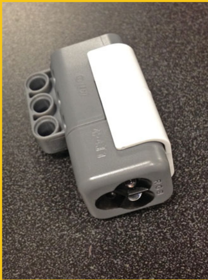
FIGURE 1.36 The color sensor is a multipurpose part that you'll find many ways to use.
