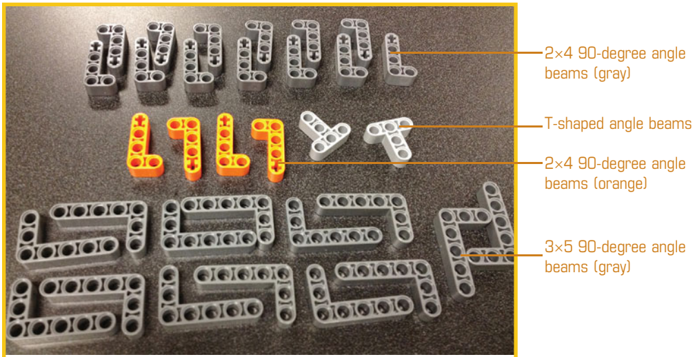
FIGURE 1.22 L- and T-shaped angle beams provide stability and provide lots of building options.
