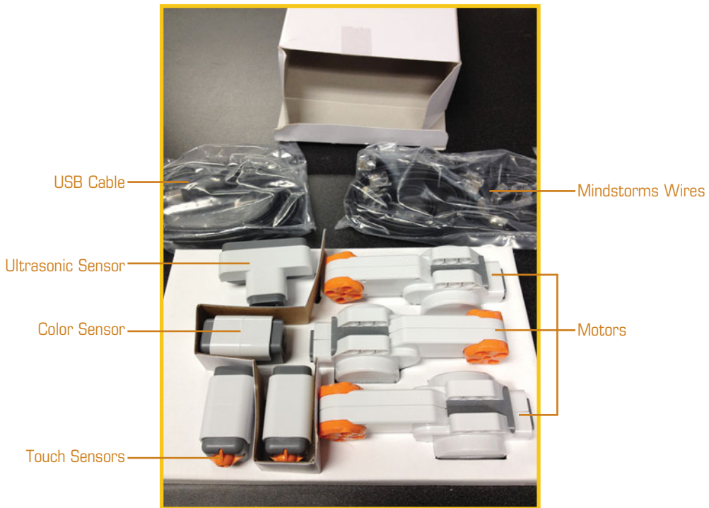
FIGURE 1.32 This box contains the sensors, motors, and wires you'll need to turn a model into a robot!
