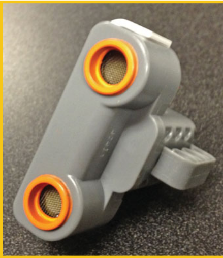
FIGURE 1.33 Ultrasonic sensors emit sound waves that help your bot measure distance.
