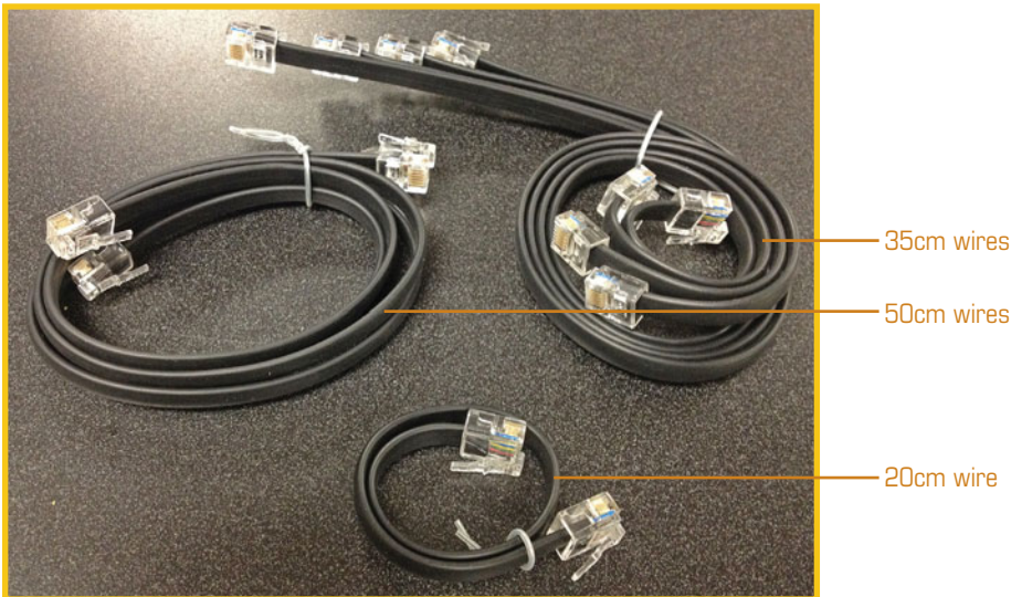
FIGURE 1.38 These wires carry the communications from the NXT brick to your bot's motors and sensors.
