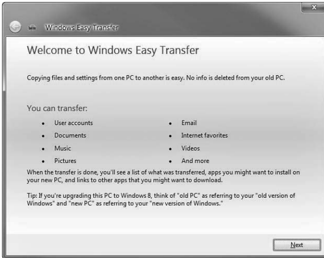
Figure 3-2 Windows Easy Transfer presents a wizard that facilitates transferring files from an old computer running Windows XP or later.
