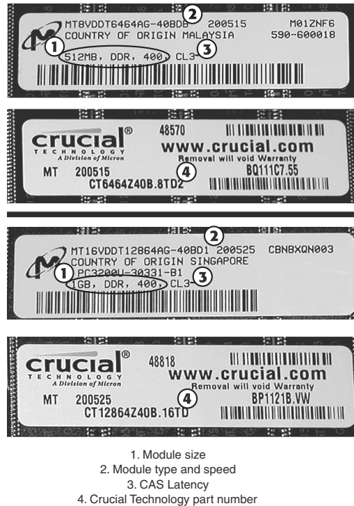
Figure 6.15 Markings on 512MB (top) and 1GB (bottom) DDR memory modules from Crucial Technology.
